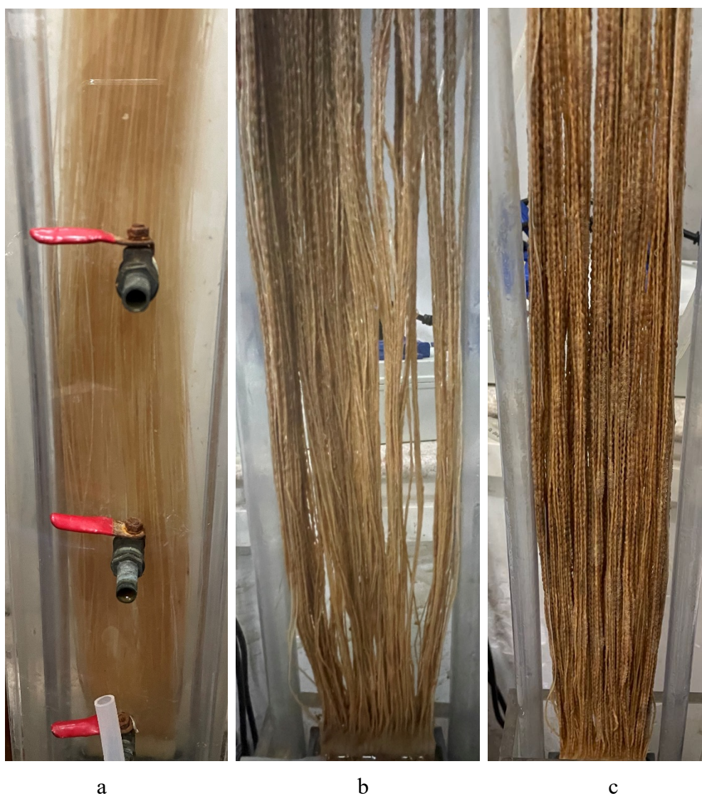
Fig. S1. Visualization of MABR biofilm with time (a. biofilm enrichment; b. HRT=8 h; c. HRT=3h)
