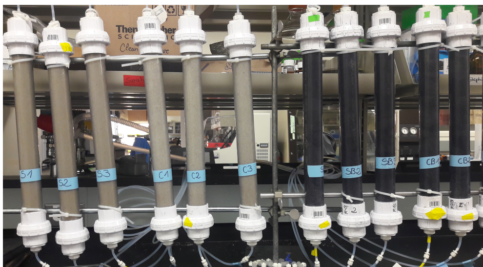
Figure S8 Laboratory column setup. Upflow columns labeled with S1-S3 contained silica sand, C1-C3 contained silica sand mixed with 20 wt% carbonate sand, SB1-SB3 contained silica sand mixed with 1 wt% MCG biochar, CB1-CB3 contained silica sand mixed with 20 wt% carbonate sand and 1 wt% MCG biochar.
