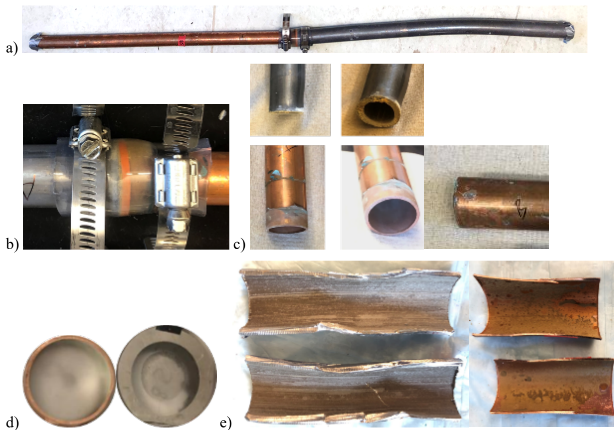
Figure S14. Example photographs of scales on a test piece exposed to synthetic water with SRNOM (TP8[pH+/DIC+/Hard+/NOM+]): a) entire length of the lead and copper pipes at end of the experiment; b) magnified photograph of the lead and copper connection; c) deposits on the ends of the lead and copper pipes near the connection and on the far end of the copper pipe; d) cross-sections of the lead and copper pipes embedded in epoxy; e) cross-sections of the lead and copper pipes.
