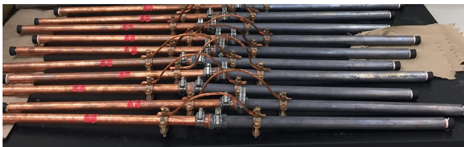
Figure S1. Lead and copper test pieces utilized in the experiment. The lead and copper pipes were attached with flexible polyvinylchloride tubing and separated using a rubber hose washer. The galvanic connection was provided using bronze ground clamps and copper ground wire.
