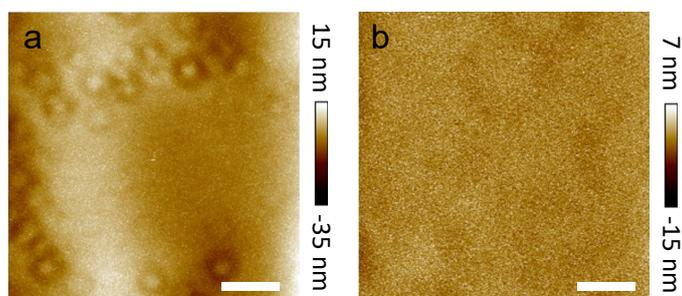
Fig. S4 (a and b) AFM images of pristine Cu(100) electrode at 2 V in 0.5 M LiTFSI/Py<sub>14</sub>TFSI-Py<sub>14</sub>FSI. Scale bars are 6 μm in (a) and 2 μm in (b).
