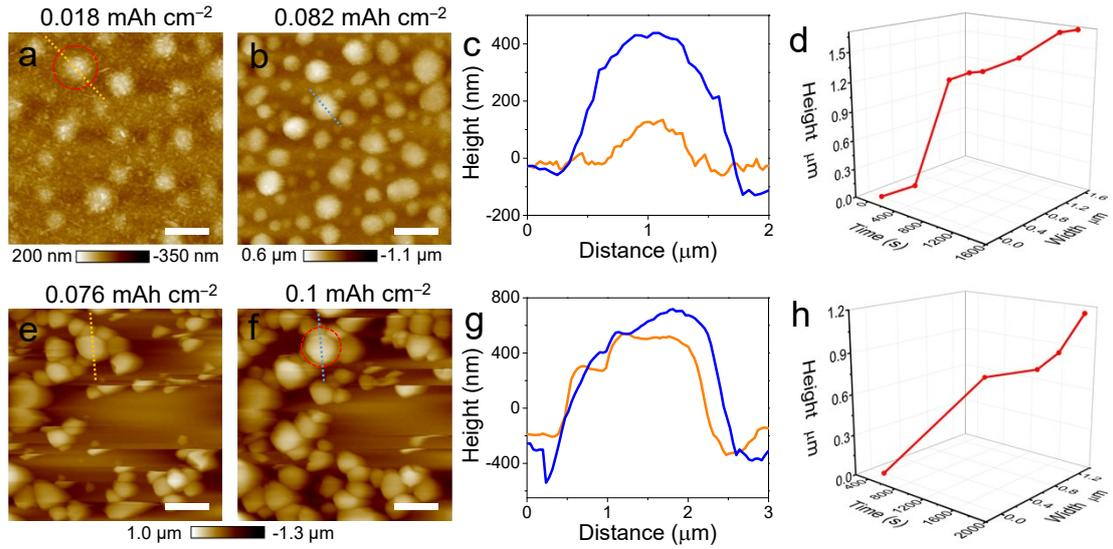
Fig. S5 In-situ AFM images of different Li deposition capacity (a, b) after SEI-Cu-lsv formation and (e, f) potential stepping from 2 V to -100 mV. (c, g) Cross section profiles of particles in (a, b) and (e, f), respectively. (d, h) Development of height and width of a growing Li nucleus marked by circle in (a) and (f), respectively. Scale bars are 1  $\mu\text{m}$  in (a) and 2  $\mu\text{m}$  in (b, e and f).
