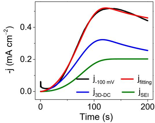
Fig. S1 The experimental current-time transient at  $-100$  mV and the corresponding theoretical current-time transient  $j_{3D-DC}$  and  $j_{SEI}$  by nonlinear curve fitting.
