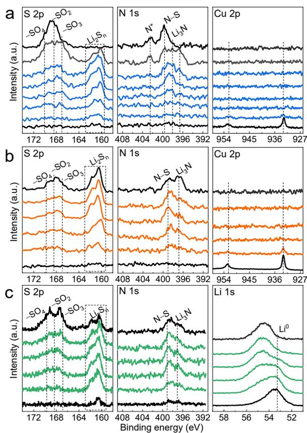
Fig. S3 XPS depth profiles of S 2p, N 1s, Cu 2p and Li 1s elements recorded after different time of argon ion sputtering at (a) SEI-Cu-lsv, (b) SEI-Cu-step and (c) SEI-Li.
