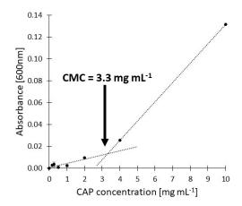
**Figure S1:** CAP absorbance at 600nm in 0.1 M KOH pH= 13.5. CAP critical micelle concentration was determined by the slope intercept at 3.3 mg mL<sup>-1</sup>.
