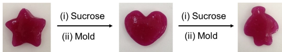
Fig. S6 Photographs showing the yeast-containing, borax-crosslinked PVA hydrogels can be simply reshaped by fuel-driven transient liquefaction.
