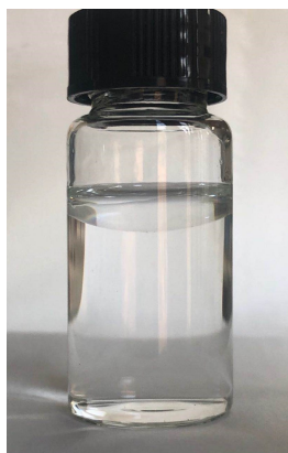
Figure S6. Photo of the APHDO product after removal of catalyst and staying at room temperature for long time. Reaction conditions: 473 K, 3.5 MPa H 2 , 12 h; 1 g pure PC pellets, 0.1 g H-USY, 0.1 g Rh/C and 40 mL H 2 O were used in the test.
