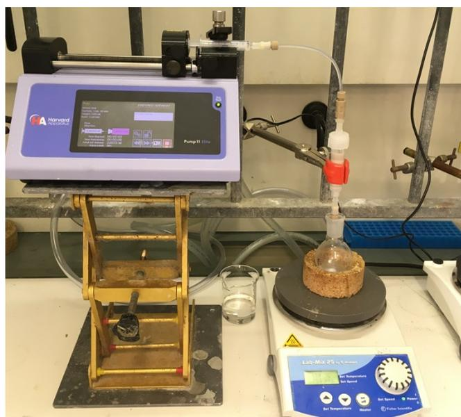
Figure 2 - Device for CEES flow neutralization with Oxone®
