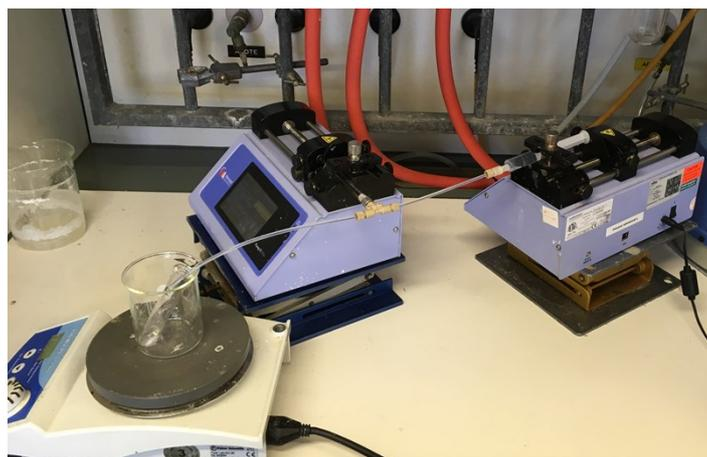
Figure 1 – Set-up for the flow neutralization of PhX with aqueous solution of  $\text{KHSO}_5$  (enriched Oxone).
