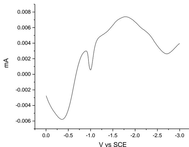
**Figure S7.** SWV of **1b** and  $\text{BF}_3 \cdot \text{Et}_2\text{O}$  using **glassy carbon** working electrode at **10 Hz**
