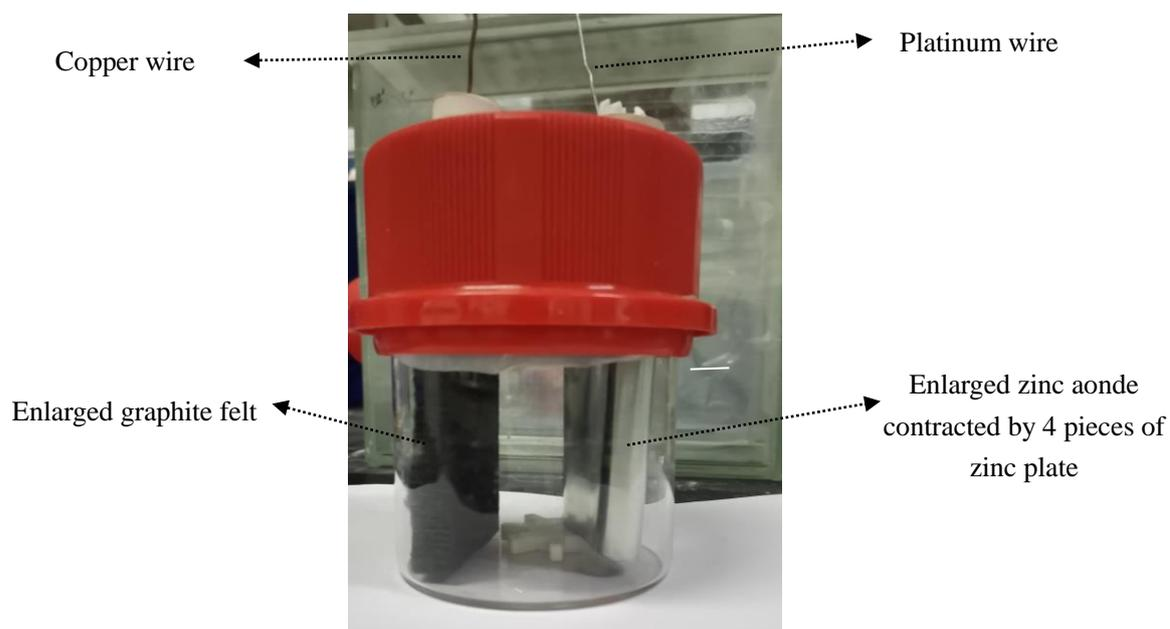
**Figure S2.** Reactor for gram scale experiment
