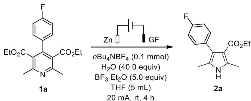
A 10 mL three-necked flask was charged with the substrate **1a** (0.8 mmol),  $n\text{Bu}_4\text{NBF}_4$  (0.1 mmol) and a magnetic stir bar. The flask was equipped with rubber stoppers, graphite felt as cathode and zinc plate as anode. The zinc plate anode attached to a platinum wire and the graphite felt cathode
