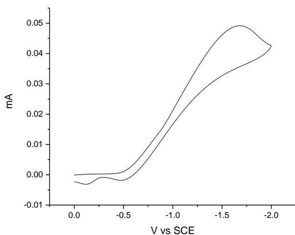
**Figure S5.** CV of **1b** using **glassy carbon** working electrode at **50 mV/s**
