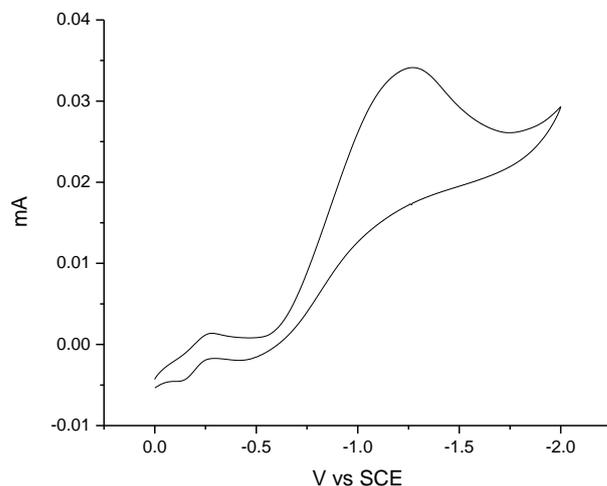
**Figure S4.** CV of **Blank** sample using **glassy carbon** working electrode at **50 mV/s**
