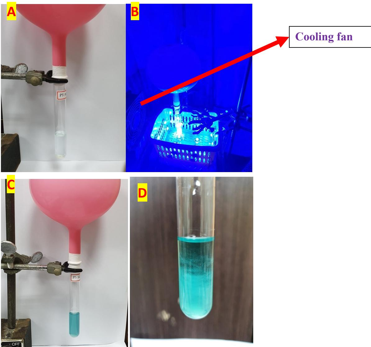
**Figure S1:** (A) Reaction mixture before irradiation. (B) Irradiation under blue LEDs, (C) & (D) Reaction mixture after irradiation showing formation of blue-colored Cu<sup>II</sup>(pic)<sub>2</sub> complex.
