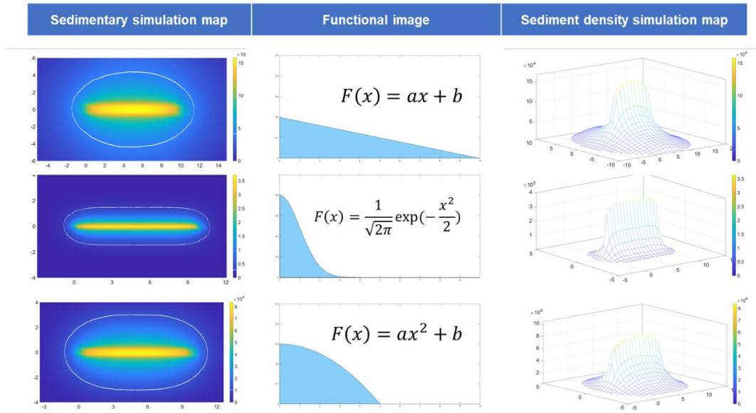
**Figure S4.** Simulation of linear PDMS deposition under different oligomers distribution patterns.
