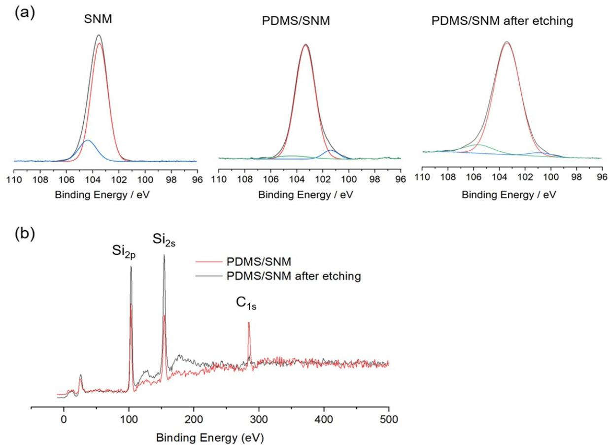
**Figure S2.** (a) Single peak fitting of Si<sub>2p</sub> for SNM, PDMS/SNM and PDMS/SNM after Ar<sup>+</sup> beam etching. (b) Si<sub>2p</sub>, Si<sub>2s</sub> and C<sub>1s</sub> Peak signal before and after etching of PDMS/SNM.
