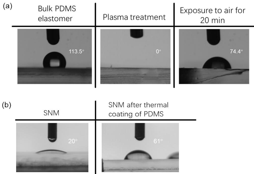
**Figure S3.** (a) The contact angle of bulk PDMS before and after plasma treatment and subsequent exposure to air. (b) The contact angle of SNM before and after conventional thermal coating of PDMS. Bulk PDMS elastomer was put on the top of the SNM with a distance of about 1 mm and heated at 100 °C for 10 h.
