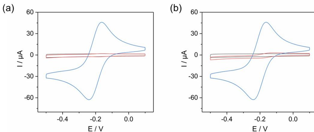
**Figure S5.** Cyclic voltammograms of p-PDMS/SNM/ITO before (black) and after (red) 4 h soaking in ethanol (a) and acetone (b) in 0.5 M KCl containing  $\text{Ru}(\text{NH}_3)_6^{3+}$ . The blue line is CV of SNM/ITO in the same solution.
