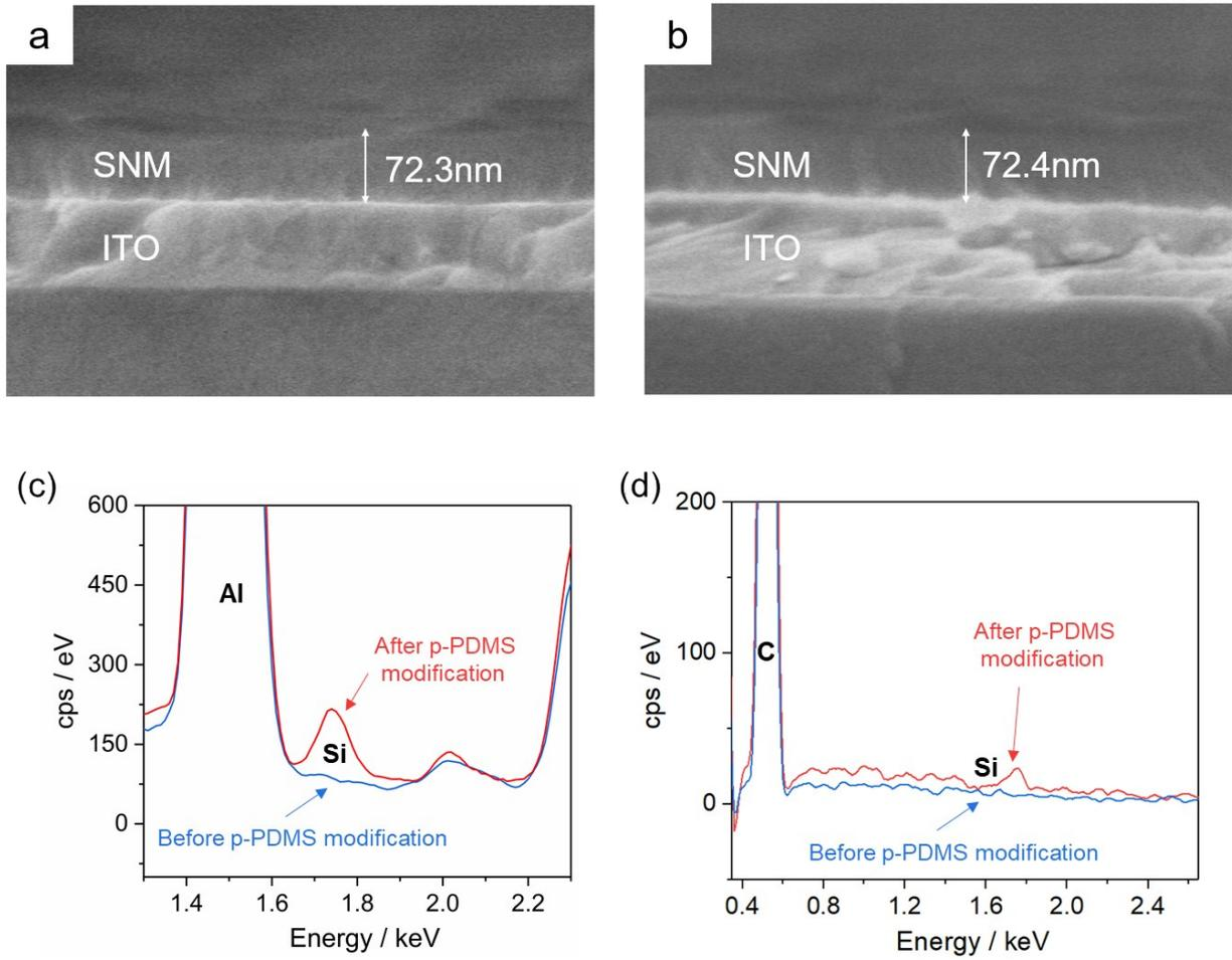
**Figure S1.** (a,b) Cross-sectional SEM images of SNM (a) and PDMS modified SNM (b). (c,d) X-ray energy spectrum of AAO (c) and PET (d) before and after p-PDMS modification.
