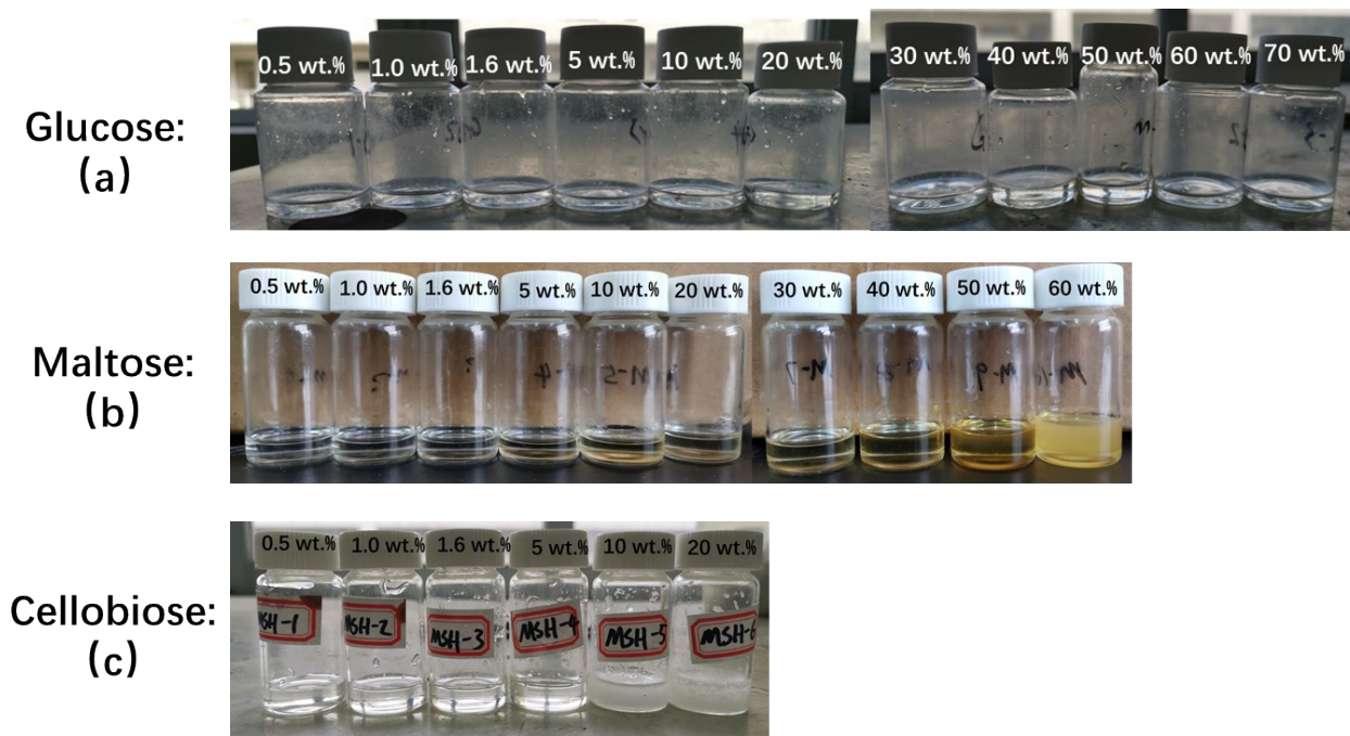
Figure S3. The morphologies of glucose, maltose and cellobiose dissolved in MSH with different concentration.
