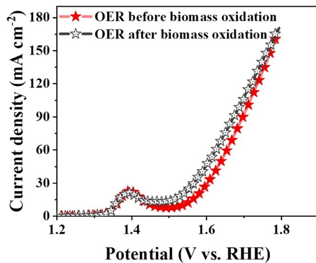
**Figure S7.** The cyclic stability test in 1 M NaOH at a sweep rate of 10 mV s<sup>-1</sup> of NiCoMn(2:1)-LDHs/NF in a four-necked round flask.
