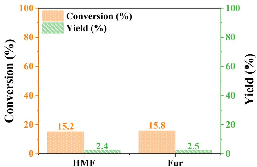
**Figure S6.** The conversion of 1 mM HMF and furfural and the yield of FDCA and FurAc at temperature of 35 °C by using pure NF.
