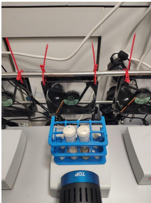
Fig. S19 Image of the setup using a single blue LED lamp.
