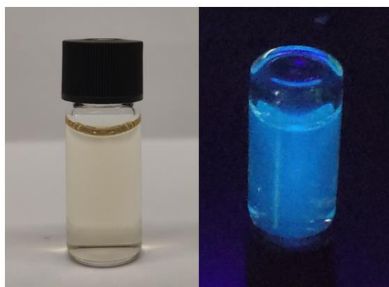
Fig. S3 Photographs of an aqueous solution of CD1 in daylight (left) and under UV light irradiation ( \lambda_{\text{ex}} = 366 \text{ nm} , right).
