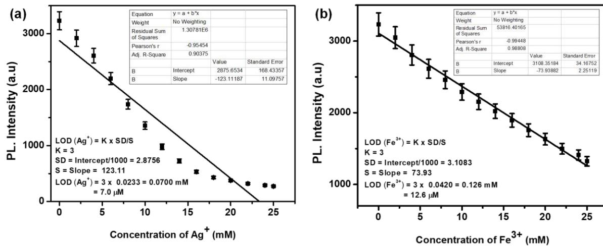
**Fig. S2.** Calibration curve of **5e** in the presence of Ag<sup>+</sup> and Fe<sup>3+</sup> ions using the monitored emission wavelength at 496 nm; (a) **5e**/Ag<sup>+</sup> and (b) **5e**/Fe<sup>3+</sup> complex systems. The detection limit (LOD) was determined from the following equation: LOD = K × SD/S, where K = 3; SD is the standard deviation
