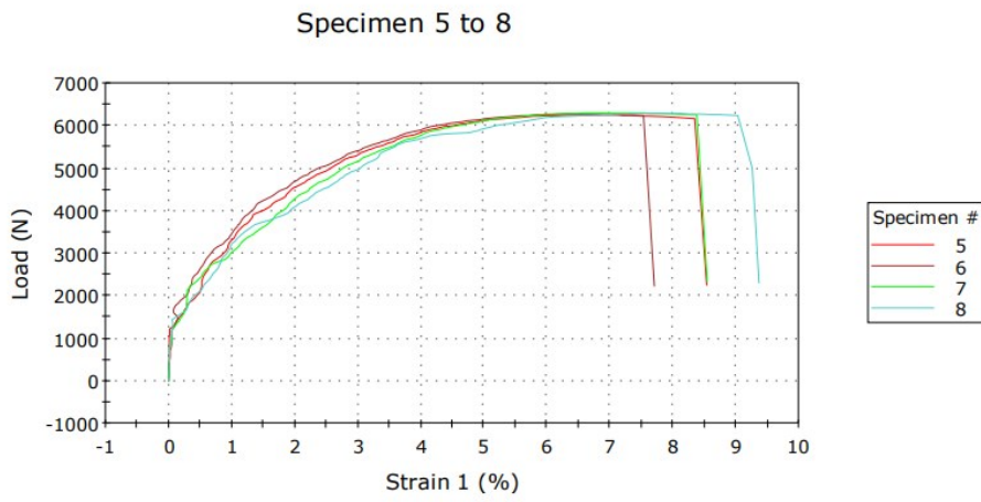
Figure S12. Stress-strain diagram of PA 612.
