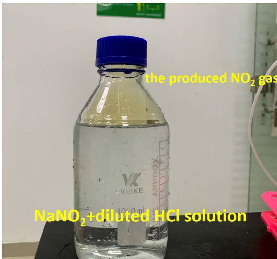
**Fig. S11.** The reaction between NaNO<sub>2</sub> and acids (such as diluted hydrochloric acid (0.1 M HCl) solution) can produce undesired nitric oxide (NO), nitrogen dioxide (NO<sub>2</sub>) contaminants.
