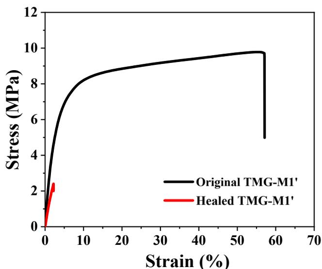
**Fig. S4** Comparison of tensile properties of the original and healed TMG-M1' samples.
