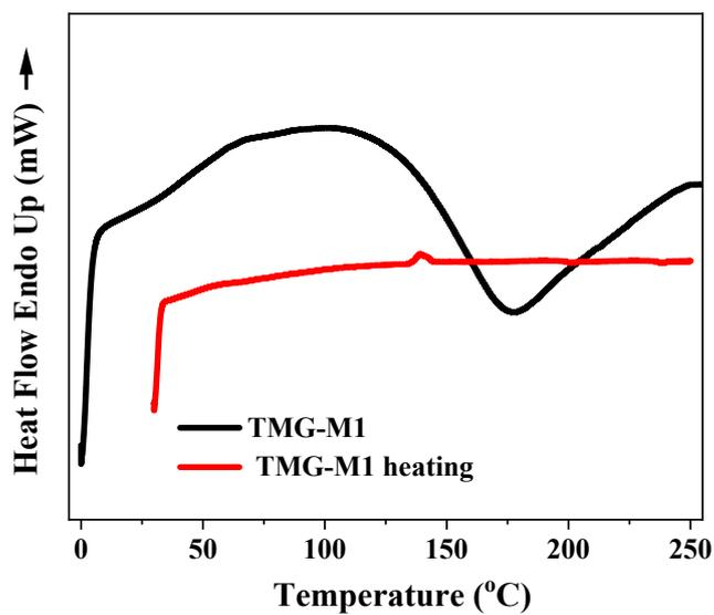
Fig. S3 DSC curves of TMG-M1 before and after heating at  $180\text{ }^{\circ}\text{C}$  for 1 h.
