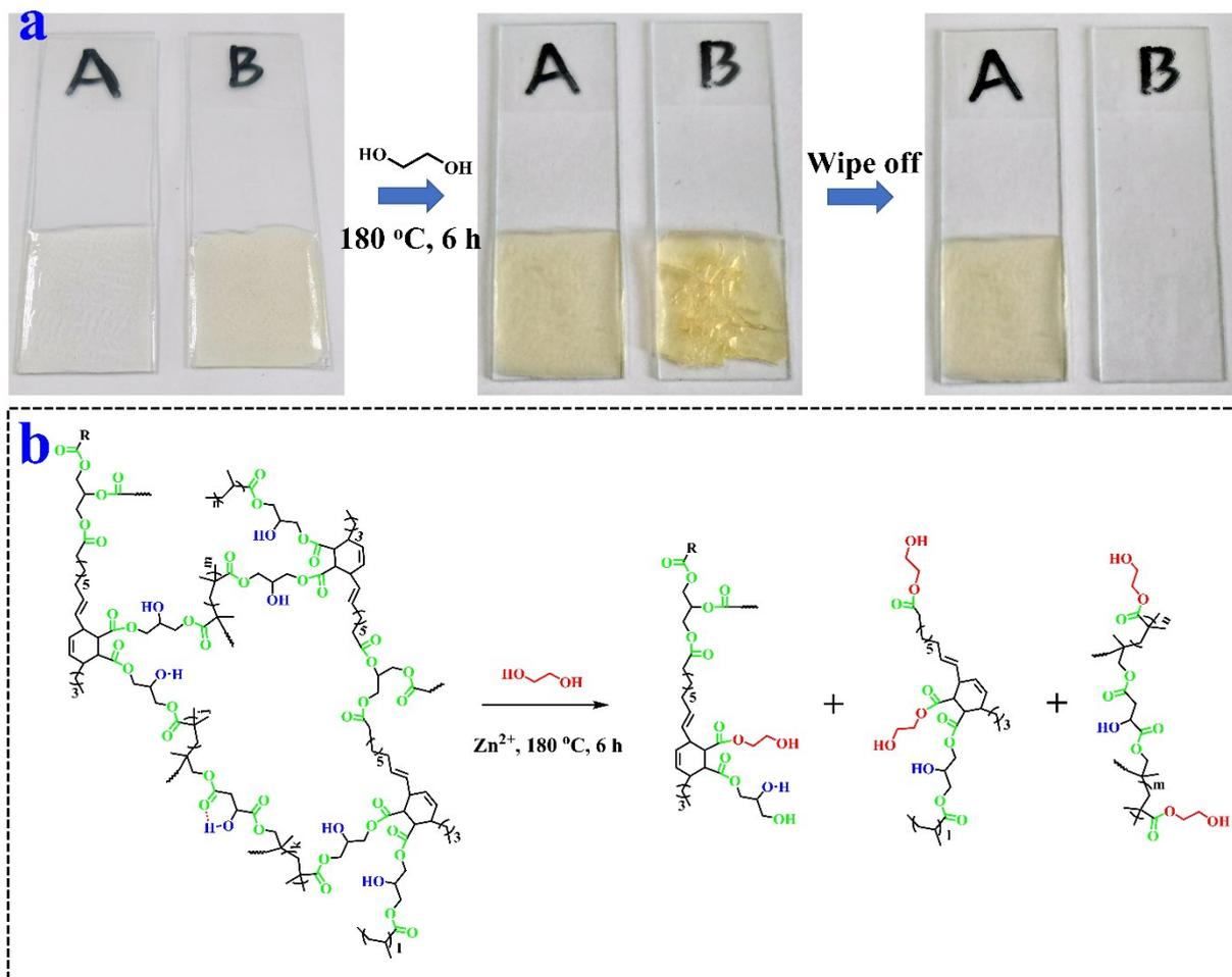
**Fig. S5** (a) Removable test of UV-cured coatings by immersing the samples (A: TMG-M1'; B: TMG-M1) into glycol solvent at 180 °C for 6 h and wiping off; (b) possible mechanism of dynamic TERs with the assistance of glycol.
