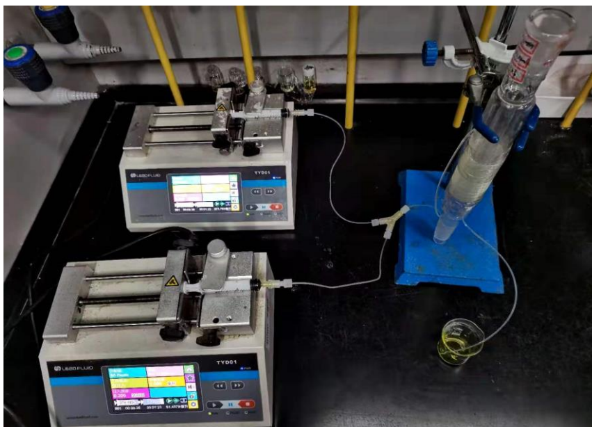
Figure S3 Details of the microreactor for the alkylation of cysteine and thioglycoside
