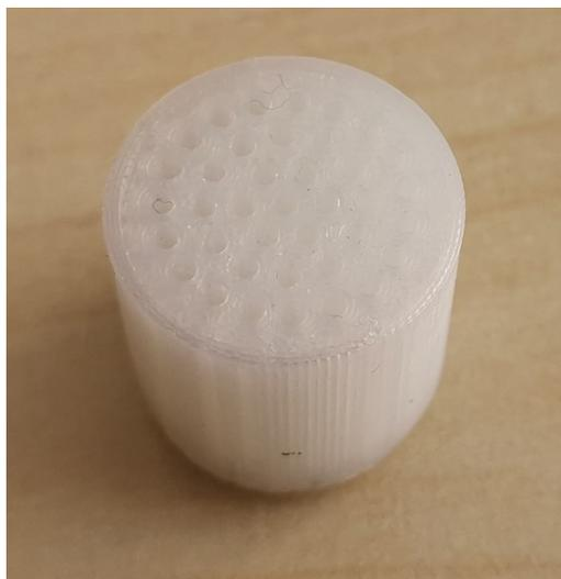
*Fig. 2 3D printed microreactor*
