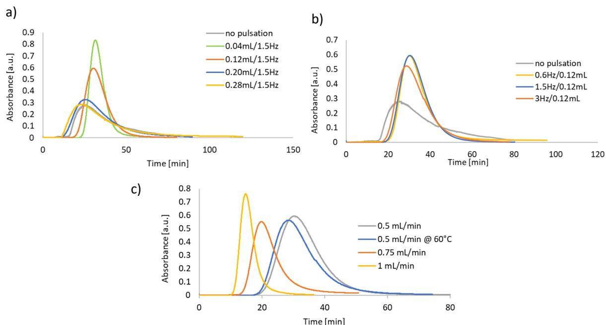
Figure S3 RTD profiles in water recorded at 563 nm. Conditions: flow rate = 500  $\mu\text{L min}^{-1}$ , 3 bar pressure, 1 mL tracer injected, 1 cm optical path length, 25 °C temperature. a) Experiments performed at 1.5 Hz pulsation frequency and different pulsation amplitudes. b) Experiments performed at different pulsation frequencies and 0.12 mL pulsation amplitude. c) Experiments performed at different flow rates (0.12 mL amplitude and 1.5 Hz Frequency, at 25°C, unless differently stated).
