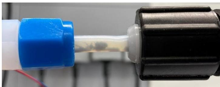
**Figure S4** Settling of Pd/Al<sub>2</sub>O<sub>3</sub> particles in the connection tubing before the pulsator pump during screening of different catalyst supports under flow conditions.
