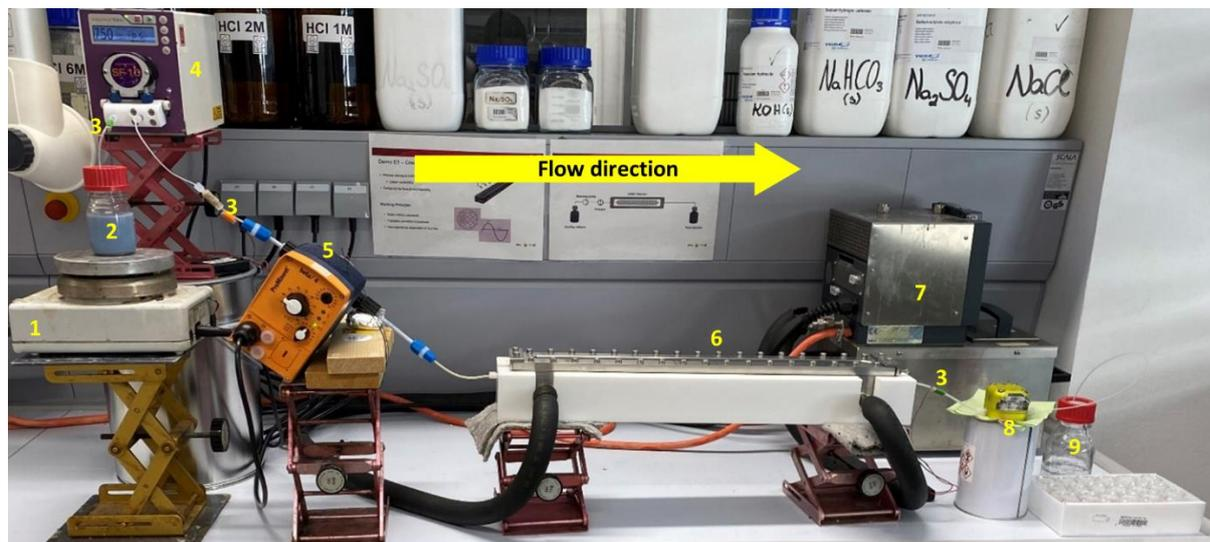
**Figure S1** Photograph of the single-feed setup used for optimization and substrate scope investigation. 1) Magnetic stirrer, 2) starting material suspension, 3) electric vibrator motors, 4) metering peristaltic pump, 5) pulsator pump, 6) HANU reactor module, 7) thermostat, 8) backpressure regulator, 9) product collection.
