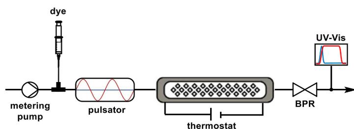
Figure S2 Schematic setup for the RTD experiments.
