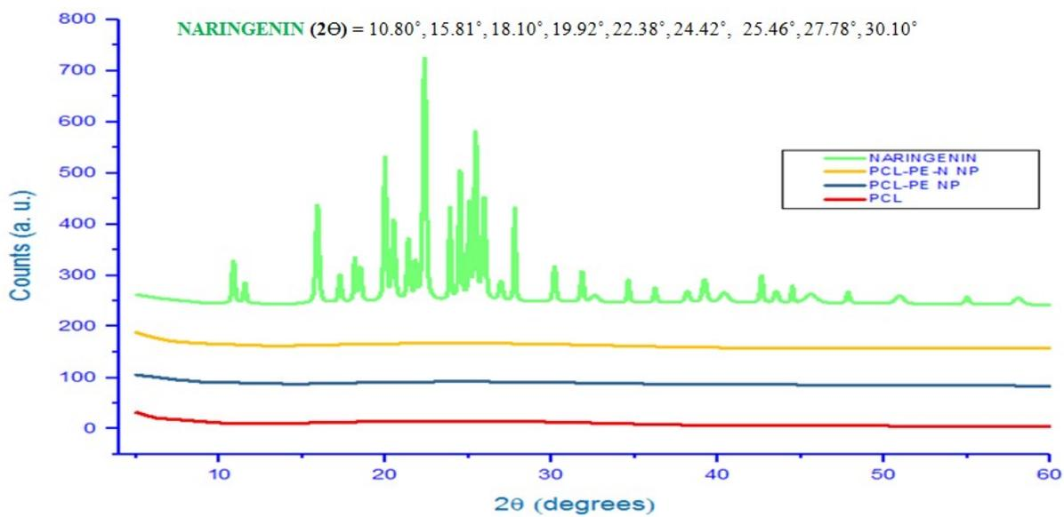
**Figure S6.** XRD pattern of PCL, PCL-PE-NPs, PCL-PE-N-NPs and pure free naringenin.
