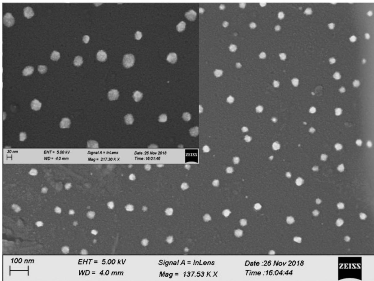
**Figure S9.** FESEM image PCL-PE-N-NPs.
