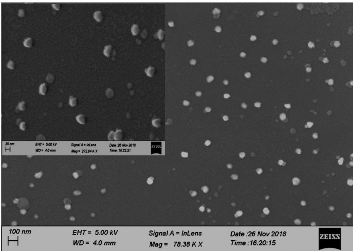
**Figure S8.** FESEM image PCL-PE-NPs.
