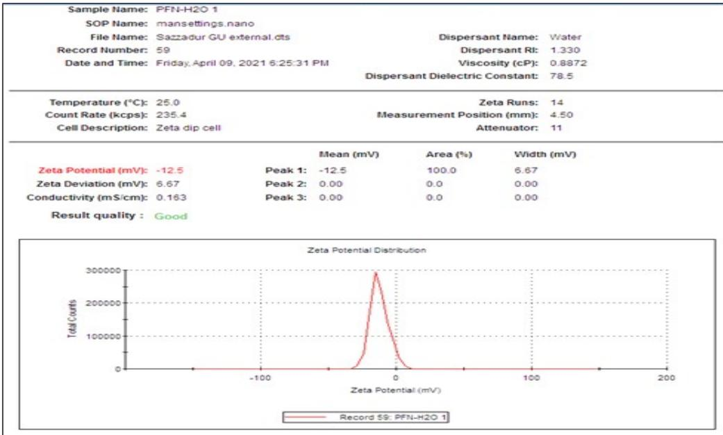
**Figure S3.** (a) Size distribution as determined by DLS , (b) Zeta potential Distribution of PCL-F68-N-NPs
