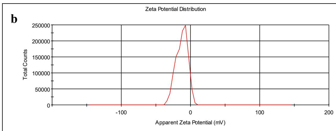
**Figure S1.** (a) Size distribution as determined by DLS , (b) Zeta potential Distribution of PCL-PE-NPs
