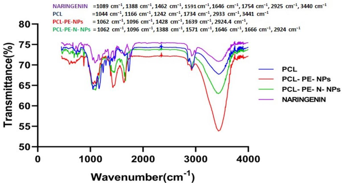
Figure S5. FTIR spectra of PCL, PCL-PE-NPs, PCL-PE-N-NPs and pure free naringenin
