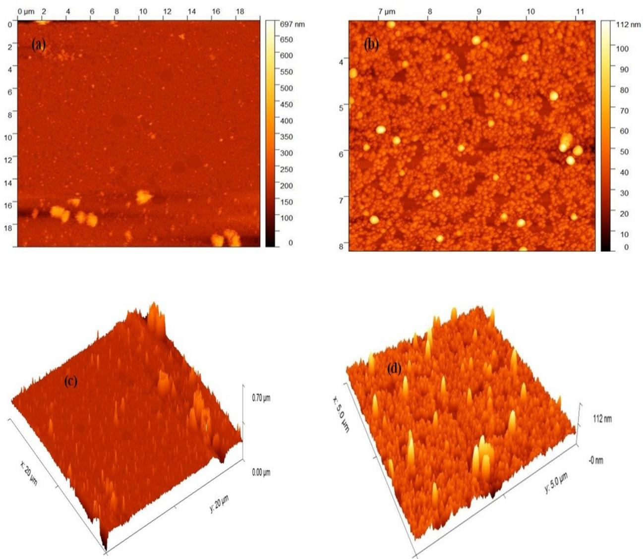
**Figure S7.** AFM 2D image (a) PCL-PE-NPs, (b) PCL-PE-N-NPs; and AFM 3D image (c) PCL-PE-NPs, (d) PCL-PE-N-NPs.
