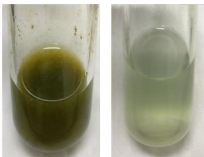
**Fig. S3. The picture after the reaction with wheat straw.** Without DMSO (left), with DMSO (right).
