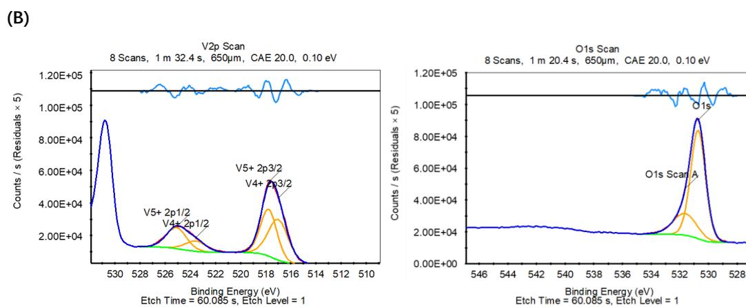
**Fig. S4. EDX (A) and XPS (B) of dark green flocculation ( $\text{VO}_2$ ).** (A) SEM-EDX mapping results of elemental distribution for V, C, O and S elements of the dark green flocculation ( $\text{VO}_2$ ). (B) V 2p (a) and O 1s (b) of XPS spectra of the dark green flocculation ( $\text{VO}_2$ ).
