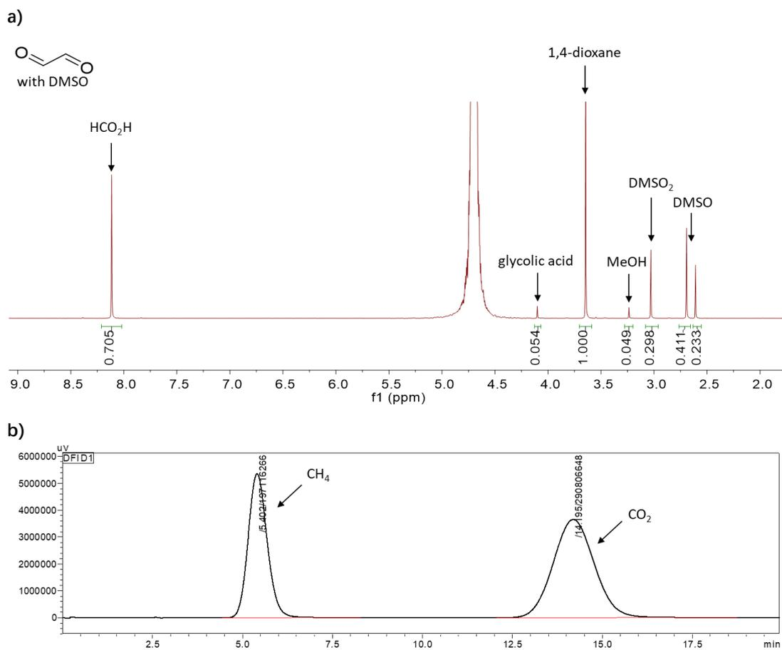
Fig. S14. <sup>1</sup>H NMR (a) and GC (b) spectra of glyoxal with DMSO sample (Table 2, entry 5).
