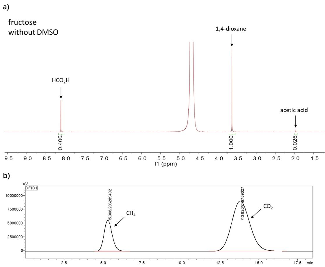
Fig. S19. <sup>1</sup>H NMR (a) and GC (b) spectra of fructose without DMSO sample (Table 2, entry 10).
