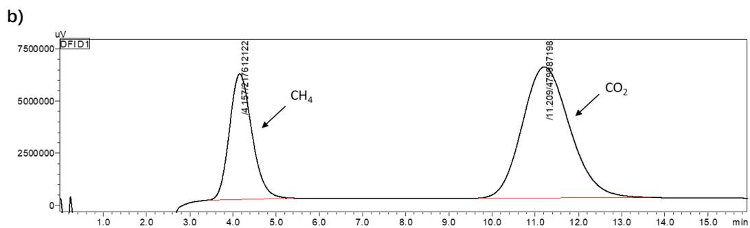
Fig. S18. <sup>1</sup>H NMR (a) and GC (b) spectra of fructose with DMSO sample (Table 2, entry 9).
