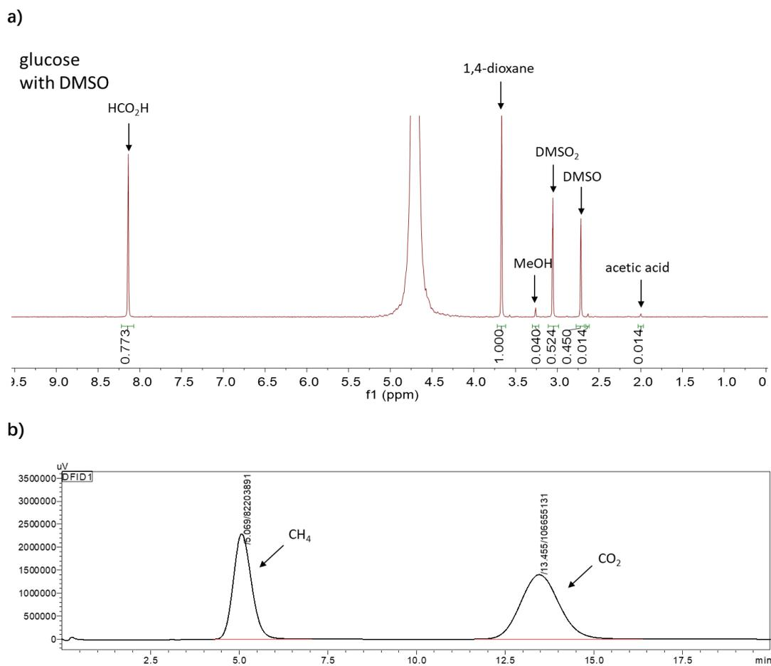
Fig. S16. <sup>1</sup>H NMR (a) and GC (b) spectra of glucose with DMSO sample (Table 2, entry 7).
