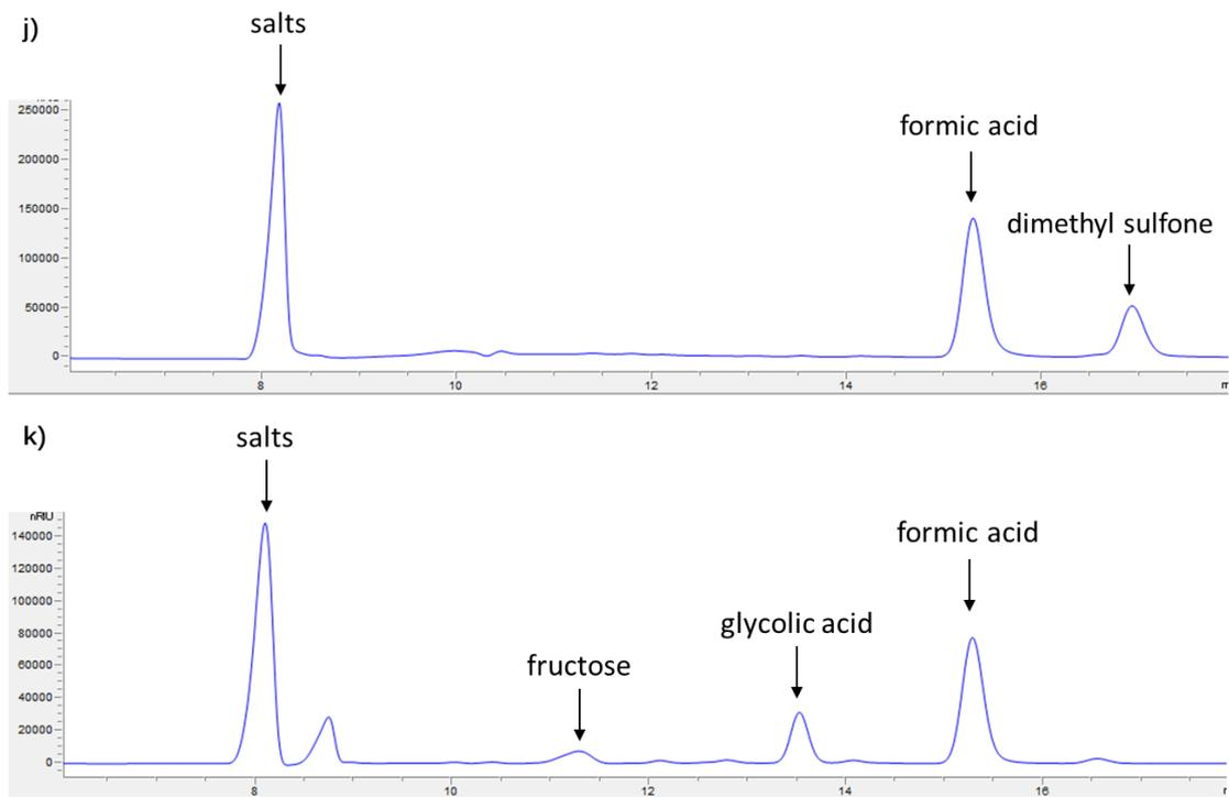
**Fig. S8. HPLC analysis of mixture after the hydrolysis–oxidation step glucose and fructose.** a)–e) glucose–without DMSO–0 min, 5 min, 10 min, 15 min to 20 min, respectively; f)–j) glucose–with DMSO–0 min, 5 min, 10 min, 15 min to 20 min, respectively; k) fructose–without DMSO–0 min.
