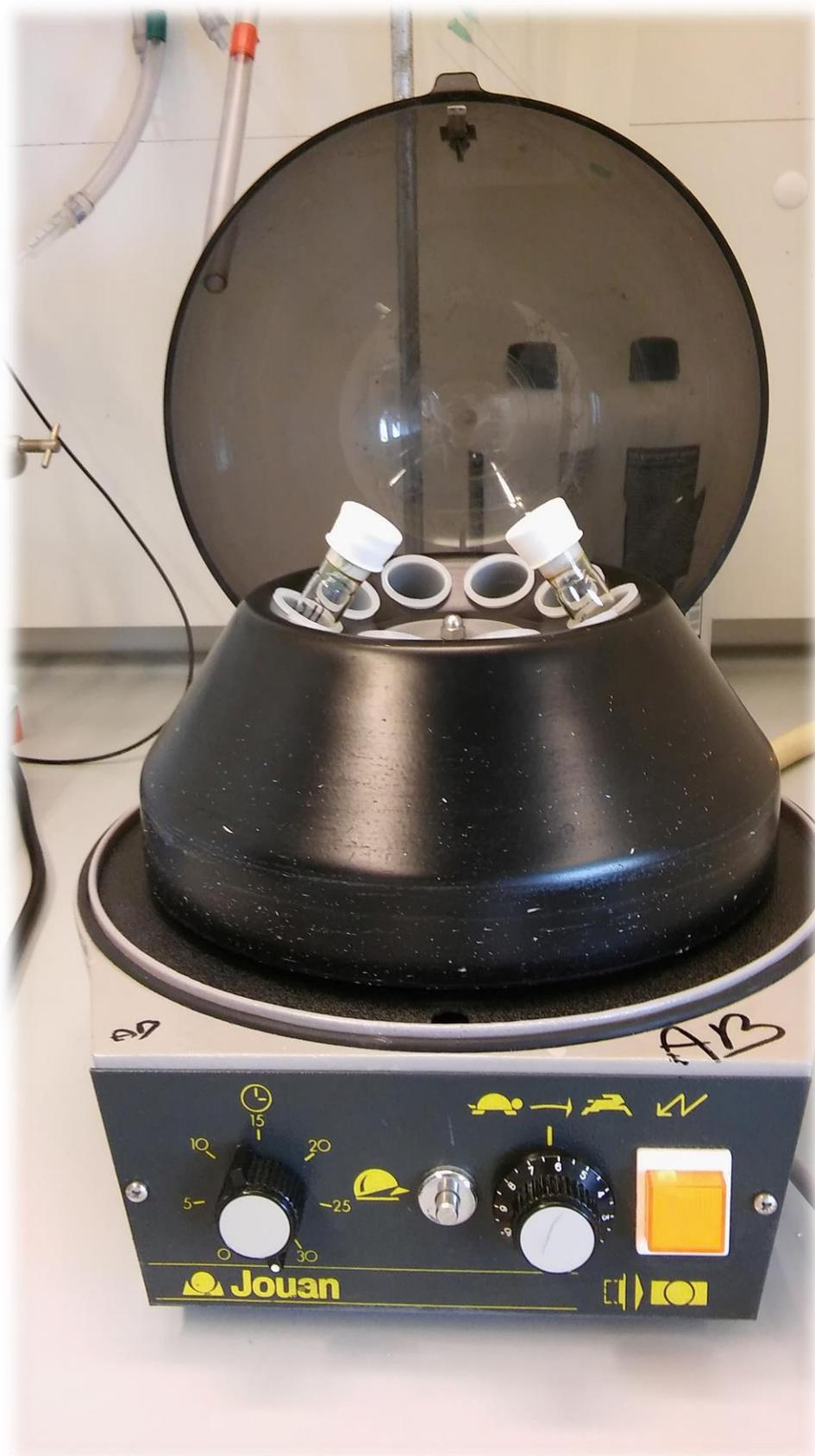
**Figure S26.** Centrifugation to precipitate inorganic matter.
