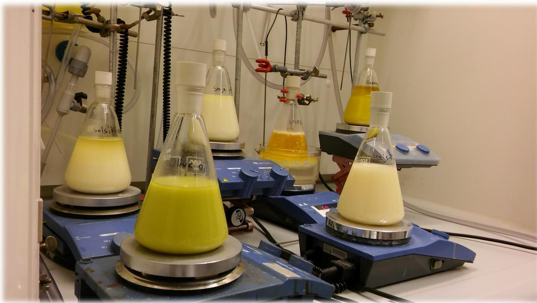
**Figure S17.** Treatment of oils with anhydrous CaCl<sub>2</sub> powder.
