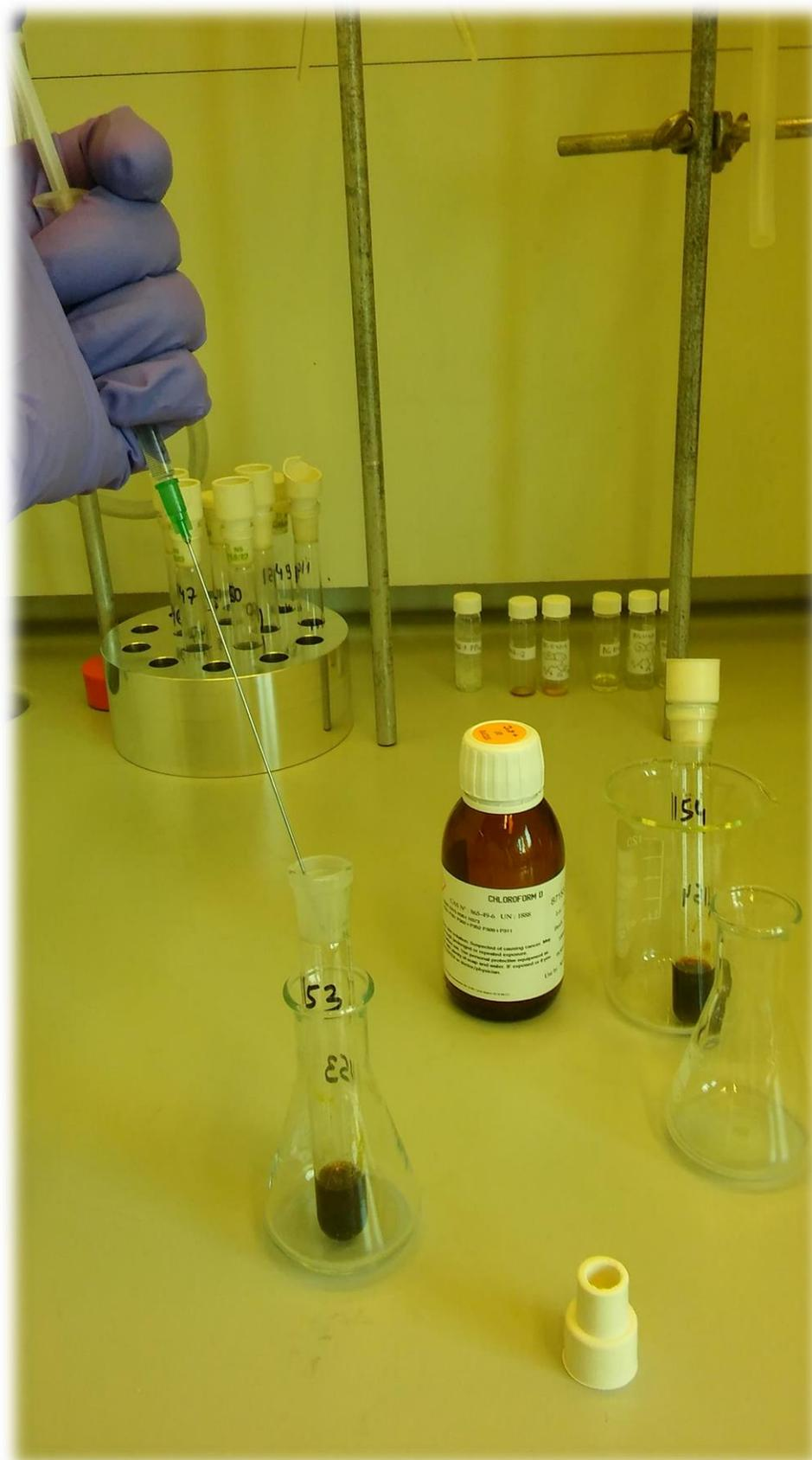
**Figure S24.** Addition of 20 drops of  $\text{CHCl}_3$  and  $\text{CDCl}_3$  (or  $\text{CCl}_4$ ).
