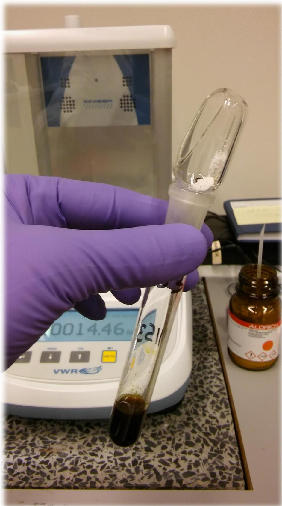
**Figure S23.** Addition of an internal standard to the reaction mixture at room temperature.
