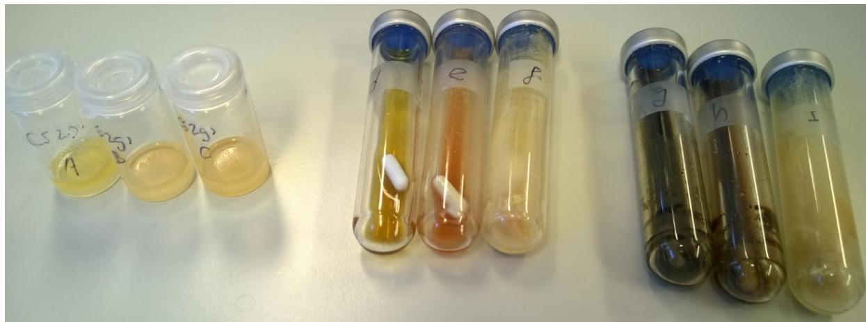
Figure SI.3.1: Photograph of decomposition studies for CPDX. Left triplet: 20°C; Middle triplet: 40°C; Right triplet: 60°C. Each triplet contains the solvents MeOH, THF, and toluene from left to right.
