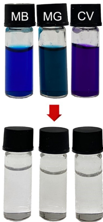
Fig. S6 Photographs of 2 mL of various dye solutions (100 mg/L) before and after filtration. MB, methylene blue; MG, methylene green; CV, crystal violet.
