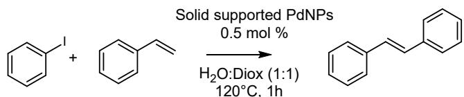
Iodobenzene (0.16 mmol), styrene (0.2 mmol) and  $K_2CO_3$  (0.32 mmol) were dissolved in a solution of H<sub>2</sub>O: 1,4-Dioxane (1:1) and 0.5 mol% of solid supported PdNPs were added. The reaction was heated for 30 min under MW irradiation at 120 °C. The crude was filtered and washed with DCM. The desired product was extracted with DCM and injected in GC and GC-MS.
