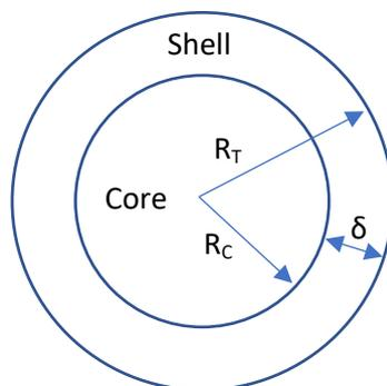
Scheme 1 – Nanoparticle core-shell structure identification of dimensions.
