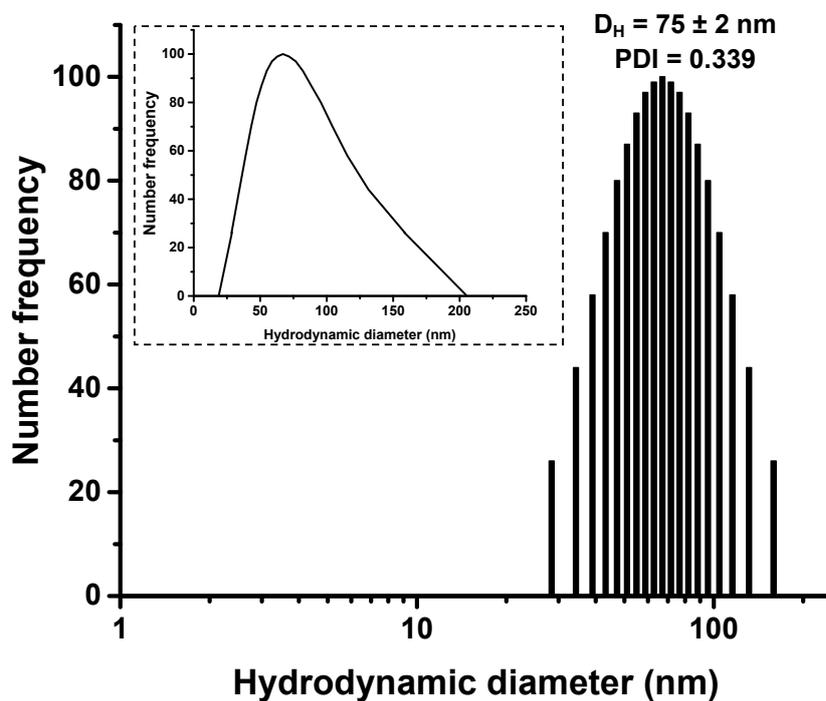
Fig. S1 Number-weighted size distribution data of AuNP-ZnS@CMC fitted with a lognormal function.
