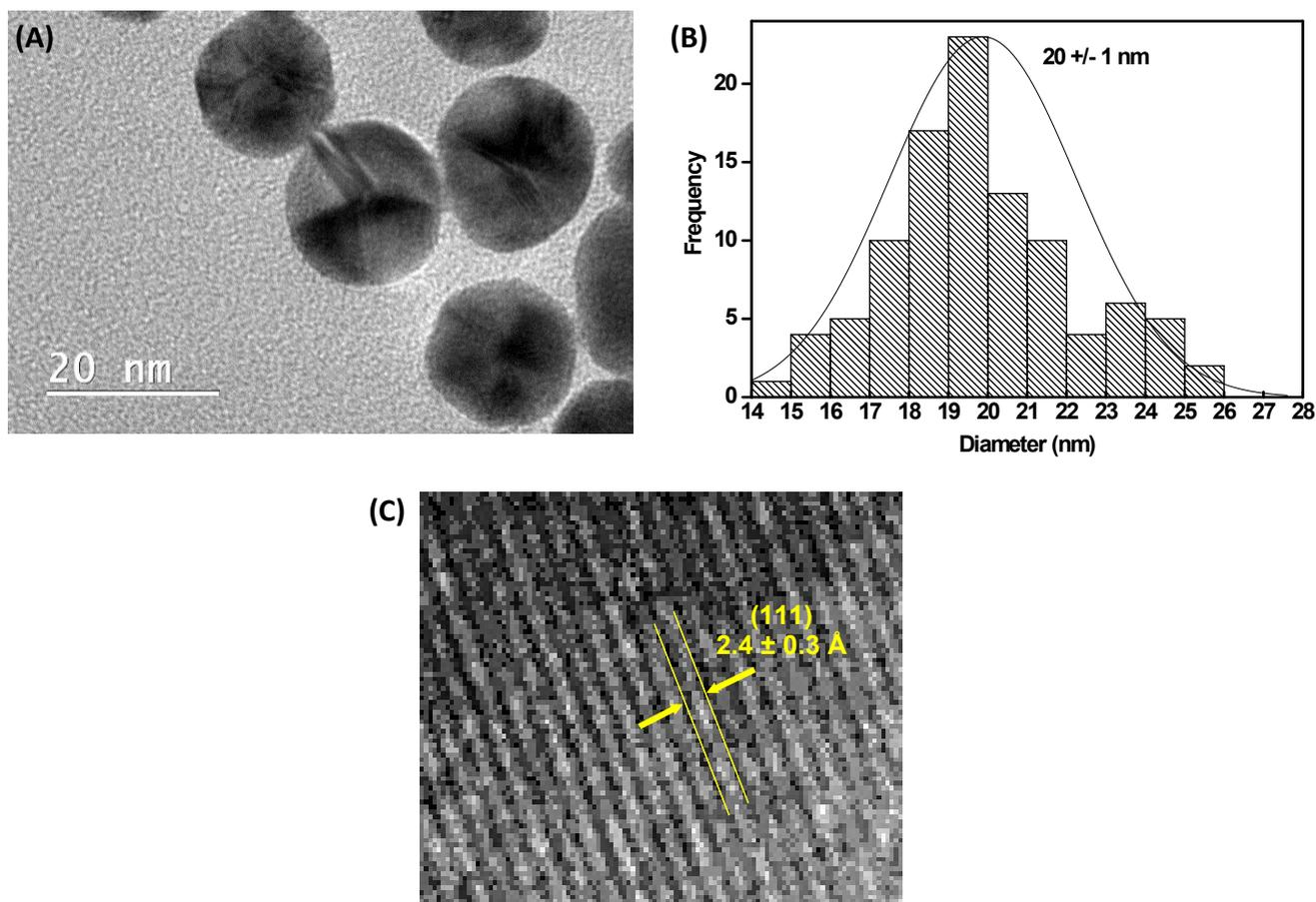
Fig. S2 (A) Transmission electron microscopy (HR-TEM) image and (B) histogram of the size distribution of AuNP@CMC. (C) Lattice fringes with interplanar distance in a high-resolution TEM image of AuNP@CMC.
