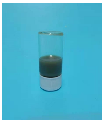
Figure S6. Free radical quenching experiments. NO gelation can be observed after KI added (0.1 g).
