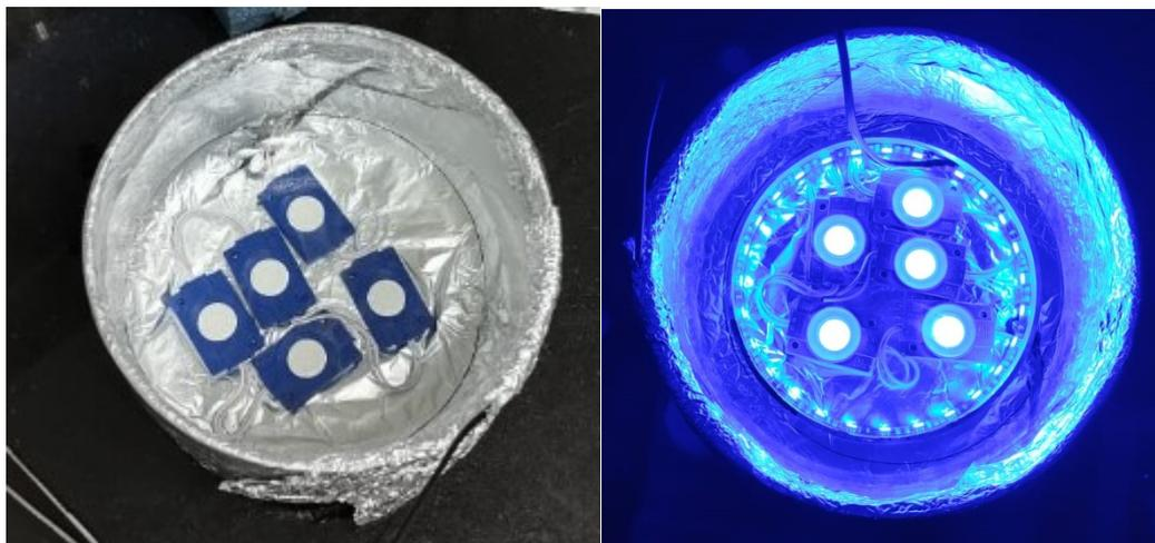
Figure SS1: Blue LED Reaction Set-up for gram scale synthesis.
