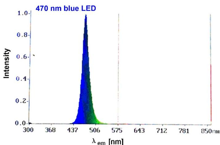
**Figure S2** Emission spectra of the used light sources.
