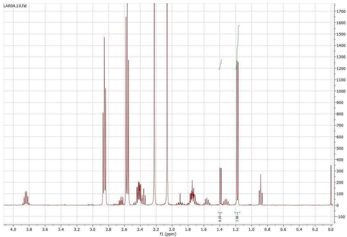
**Figure S6.**  $^1\text{H}$  NMR spectrum for electrolysis performed in 0.1 M acetate buffer + 0.1 M  $\text{KClO}_4$  at -1.9 V vs. RHE, for 4 F/mol of LA.
