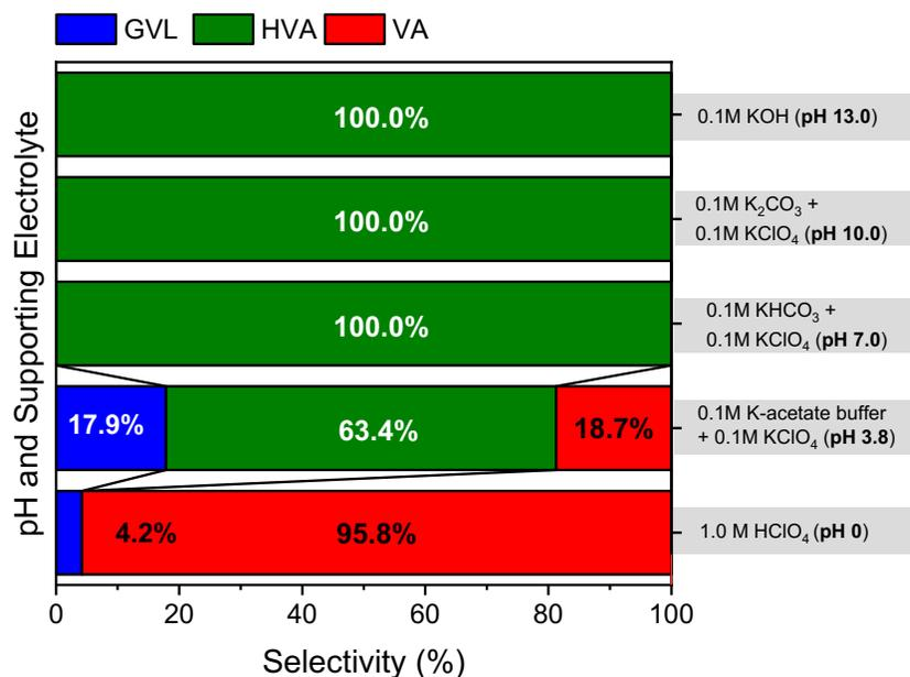
**Figure S4.** pH and supporting electrolyte effect on selectivities for electrolyses performed with 0.1 mol L<sup>-1</sup> LA, at -1.9 V vs. RHE, for 4 F/mol of LA. VA: valeric acid, HVA: 4-hydroxyvaleric acid, GVL:  $\gamma$ -valerolactone, and FA: formic acid.
