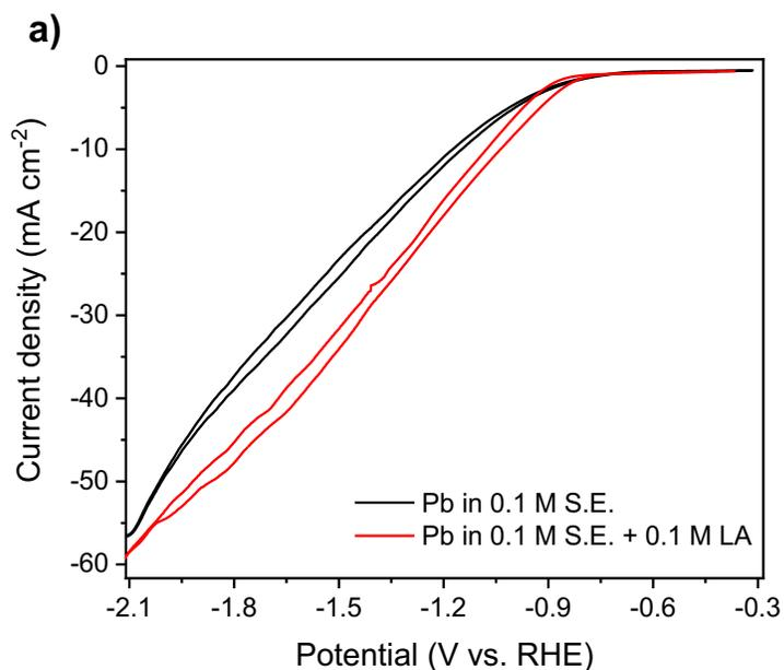
**Figure S9.** Cyclic voltammograms of Pb electrode in 0.1 M KHCO<sub>3</sub> + 0.1 M KClO<sub>4</sub> (pH 7), with and without 100 mM levulinic acid at a scan rate of 50 mV s<sup>-1</sup> and 20°C.
