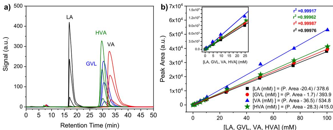
**Figure S2.** a) Chromatograms for different concentrations of LA, VA, GVL, and HVA, using UV detector at 210 nm, column temperature of 60 °C, flow rate of 0.4 mL min<sup>-1</sup>, and 12.5 mM H<sub>2</sub>SO<sub>4</sub> as eluent. b) Calibration curves.
