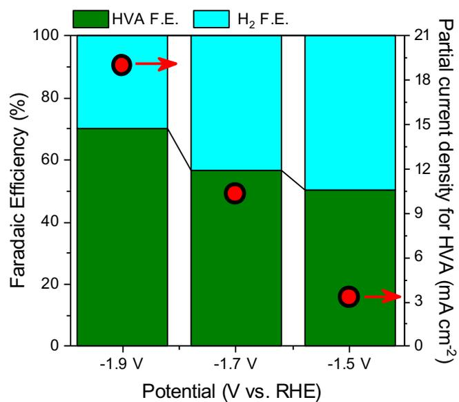
**Figure S10.** Potential effect for electrolyses carried out at 50 °C, with 2 F/mol of LA in 0.1 M KHCO<sub>3</sub> + 0.1 M KClO<sub>4</sub>.
