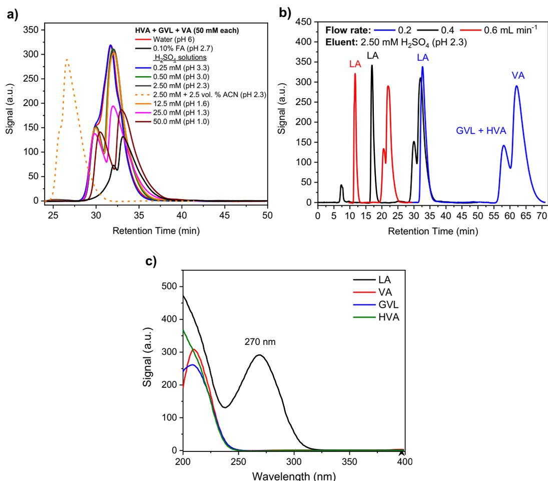
**Figure S1.** Chromatograms for a mixture of 50 mM LA, VA, GVL, and HVA, using UV detector at 210 nm and column temperature of 60 °C. **a)** Eluent effect: flow rate of 0.4  $\text{mL min}^{-1}$  and different eluents. **b)** Flow rate effect: 2.50 mM  $\text{H}_2\text{SO}_4$  as eluent and flow rates of 0.2, 0.4, and 0.6  $\text{mL min}^{-1}$ . **c)** UV-vis spectra for LA, VA, GVL and HVA.
