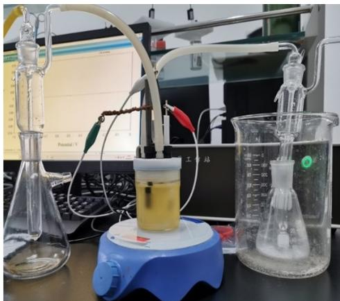
**Figure S12.** Experimental apparatus of the electrochemical reduction of  $N_2$  to  $NH_3$ .
