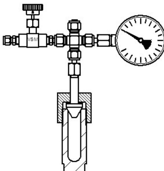
Figure 1: Schematics of the used high pressure reactors (digital manometers were used to record the pressure-curves).
