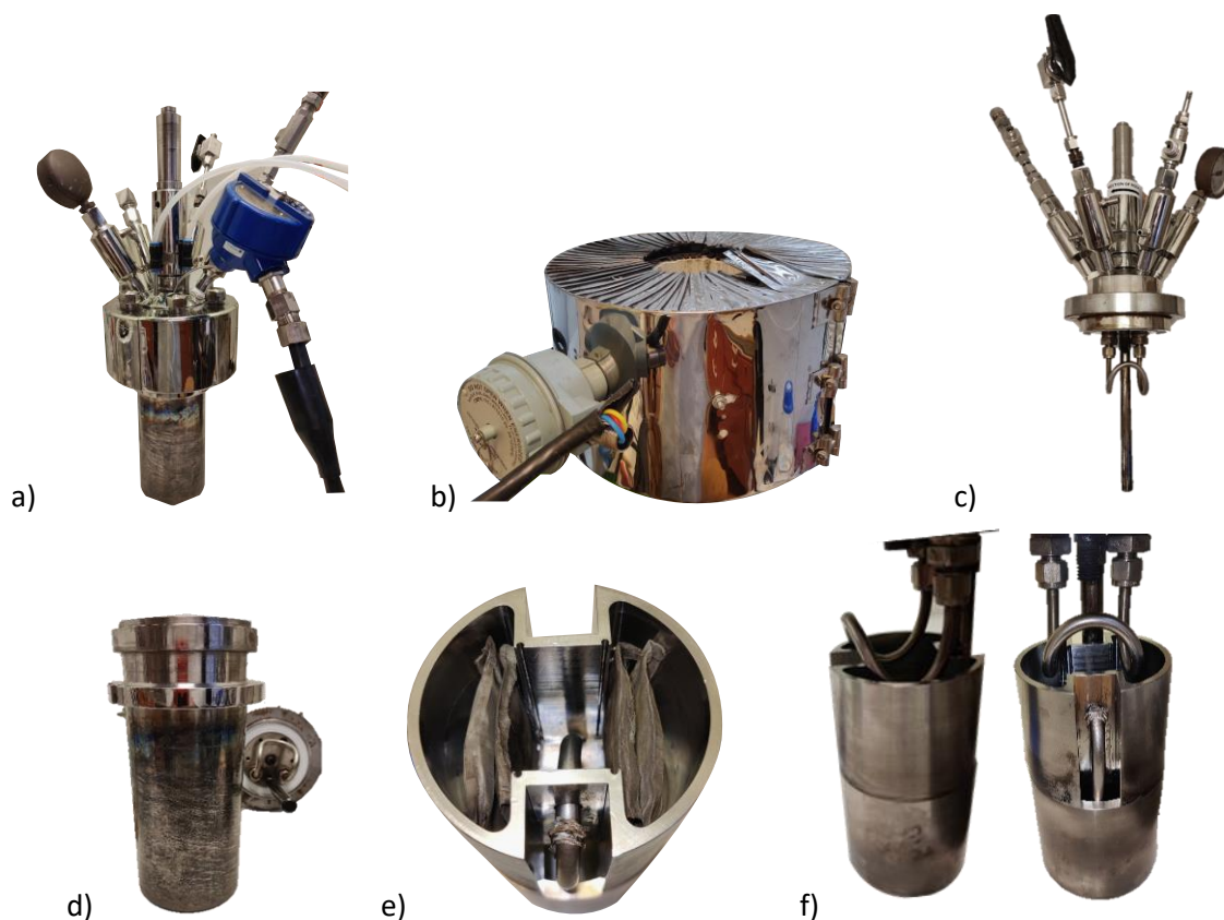
Figure S3 Pictures of the reactor system. a) picture of the assembled reactor; b) heating unit; c) reactor head bearing the pressure valve, pressure gauge, burst valve, cooling coil, and thermowell; d) 600 mL reactor vessel and reactor head showing the PTFE white gasket; e) EC showing the syphon and the substrate wrapped in steel net; f) reactor head positioned on top of EC and CC simulating the assembled reactor.
