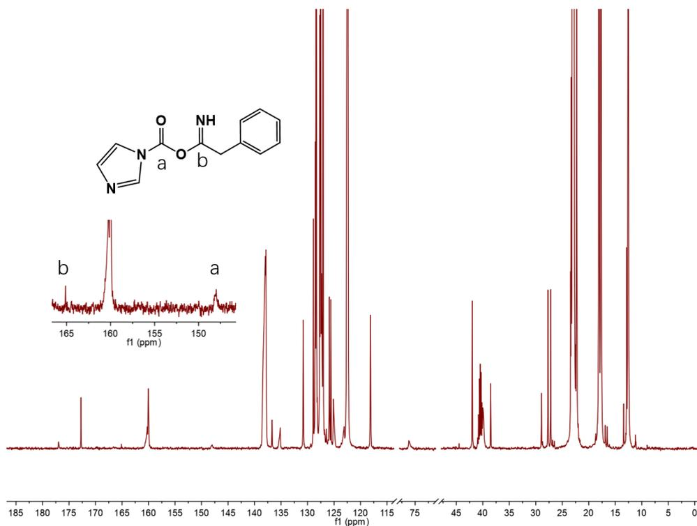
**Figure S10.** *In-situ*  $^{13}\text{C}$  NMR spectrum for the reaction solution of **1a** hydration over  $[\text{P}_{4444}][\text{Im}]$  performed at  $90^\circ\text{C}$  for 4 h.
