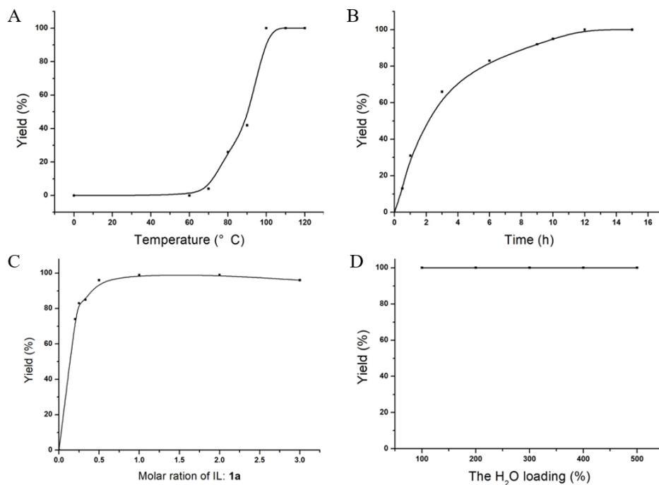
**Figure S13.** Effects of reaction factors on the product yields. Reaction conditions: **1a** (1 mmol) and CO<sub>2</sub> atmosphere; (a) [P<sub>4444</sub>][2-OP] (1 mmol), H<sub>2</sub>O (1 mmol), 12 h; (b) [P<sub>4444</sub>][2-OP] (1 mmol), H<sub>2</sub>O (1 mmol), 100 °C; (c) H<sub>2</sub>O (1 mmol), 100 °C, 12 h; (d) [P<sub>4444</sub>][2-OP] (1 mmol), 100 °C, 12 h.
