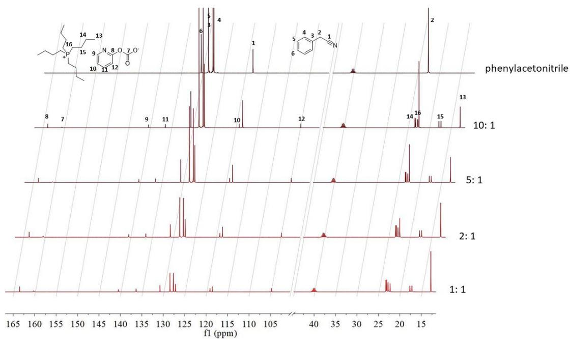
**Figure S5.** <sup>13</sup>C NMR spectra of **1a** and the mixtures of **1a**+ [P<sub>4444</sub>][2-OP] with different **1a**: IL ratios under CO<sub>2</sub> atmosphere at 70 °C.
