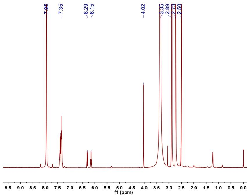
**Figure S12.**  $^1\text{H}$  NMR spectrum of the reaction solution of **1a** hydration over  $[\text{Na}][2\text{-OP}]$ .
