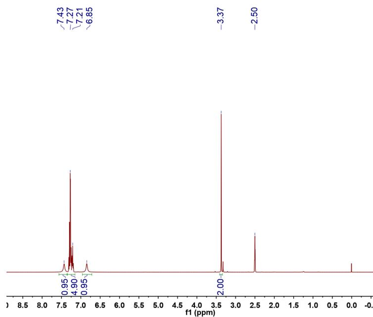
**Figure S14.** <sup>1</sup>H NMR spectrum of the product for **1a** Gram-scale reaction. Reaction conditions: **1a** (10 mmol), [P<sub>4444</sub>][2-OP] (10 mmol), H<sub>2</sub>O (10 mmol), 100 °C, 12 h, CO<sub>2</sub> atmosphere.
