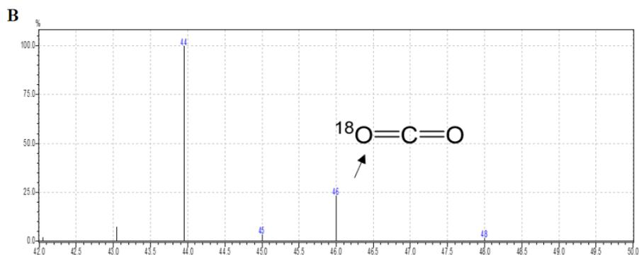
**Figure S2.** GC-MS spectra of the product from phenylacetone nitrile hydration in the presence of CO<sub>2</sub>. (A) Phenylacetamide (2a). (B) CO<sub>2</sub>. Reaction conditions: phenylacetone nitrile (**1a**, 1 mmol), [P<sup>4444</sup>][2-OP] (1 mmol), H<sub>2</sub><sup>18</sup>O (1 mmol), 100 °C, 12 h, CO<sub>2</sub> atmosphere.
