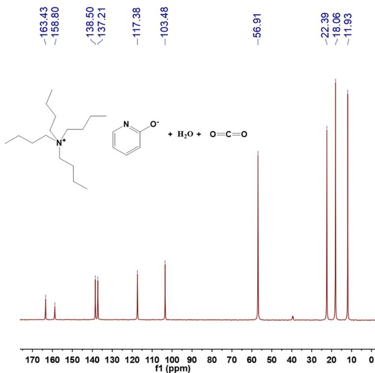
**Figure S11.**  $^1\text{H}$  and  $^{13}\text{C}$  NMR spectra of  $[\text{N}_{4444}][2\text{-OP}] + \text{H}_2\text{O}$  and  $[\text{N}_{4444}][2\text{-OP}] + \text{H}_2\text{O} + \text{CO}_2$  at  $90\text{ }^\circ\text{C}$ .
