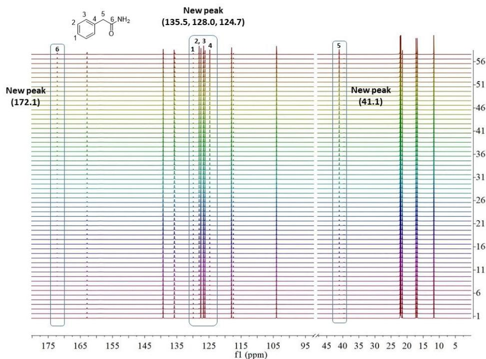
**Figure S7.** *In-situ*  $^{13}\text{C}$  NMR spectra of the reaction solutions of **1a** hydration over  $[\text{P}_{4444}][2\text{-OP}]$  at  $90^\circ\text{C}$ .
