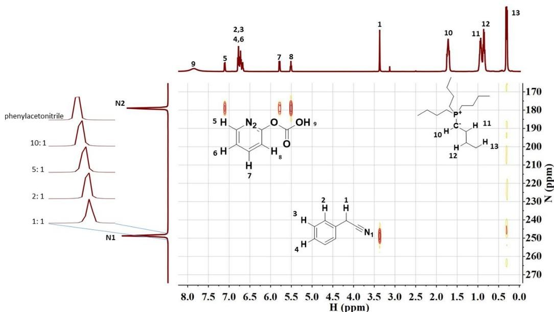
**Figure S6.**  $^1\text{H}$ - $^{15}\text{N}$  HMBC spectra of **1a** and the mixtures of **1a**+ $[\text{P}_{4444}][2\text{-OP}]$  with different ratios under  $\text{CO}_2$  atmosphere at  $70^\circ\text{C}$ .
