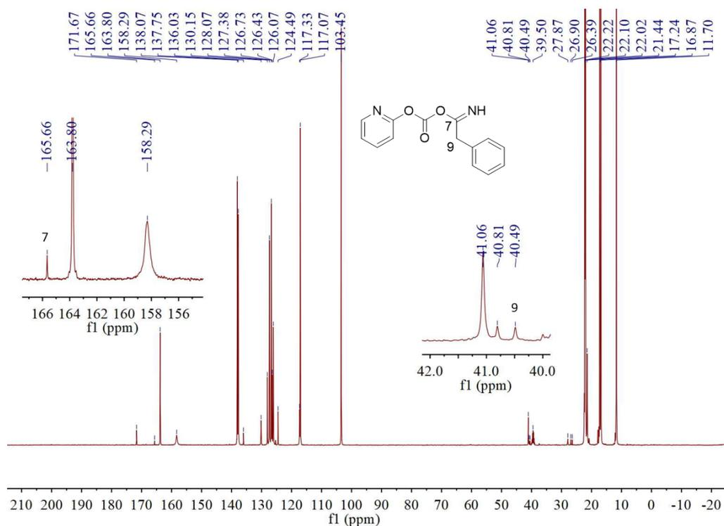
**Figure S8.** *In-situ*  $^{13}\text{C}$  NMR spectrum of the reaction system of 1a hydration over  $[\text{P}_{444}][2\text{-OP}]$  performed at 90 °C for 4 h.
