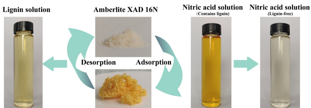
Fig. S5 Amberlite XAD16N adsorbs lignin in \text{HNO}_3 .
