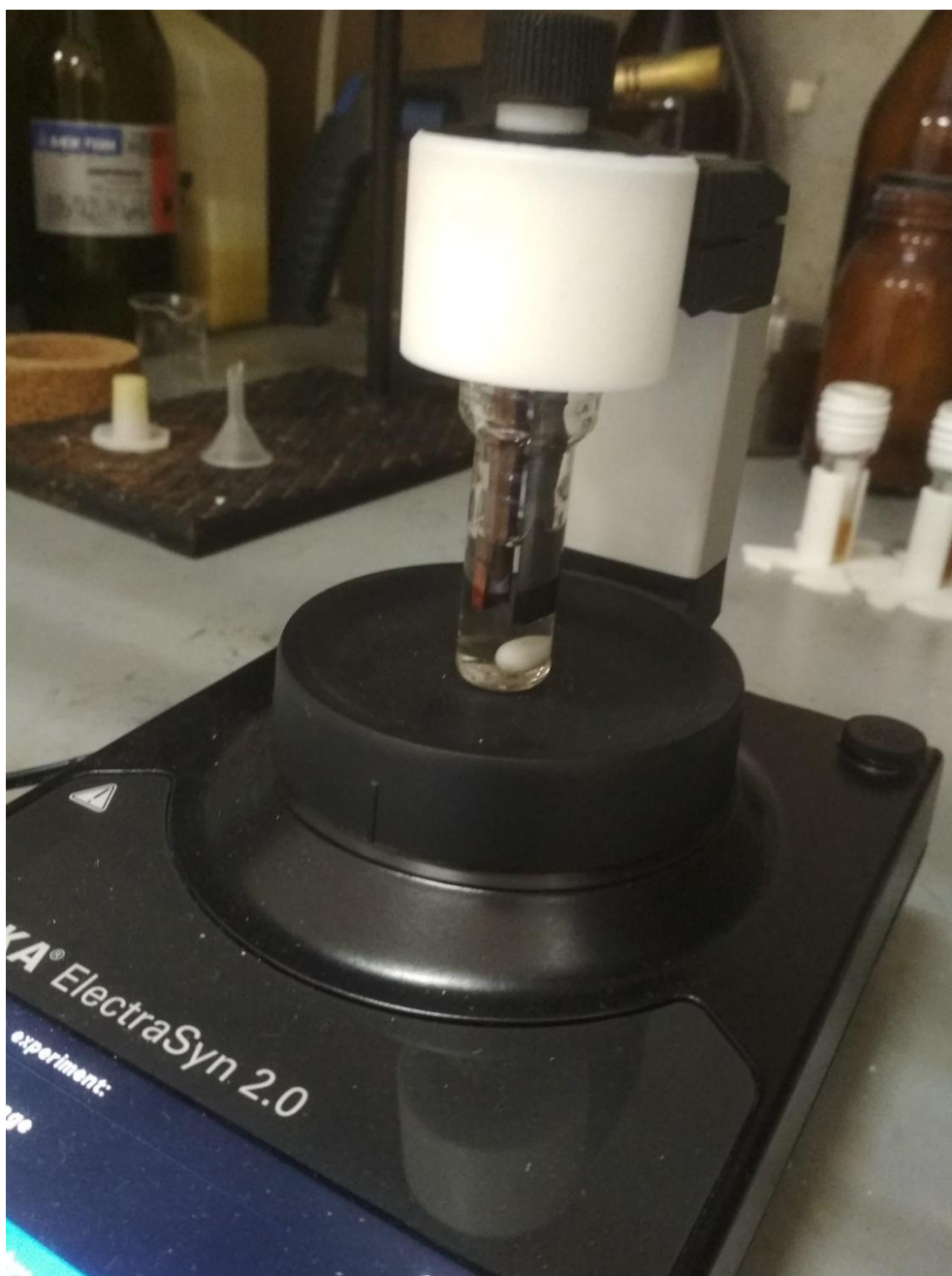
Figure S47. ElectraSyn device equipped with a single vial with two standard electrodes.
