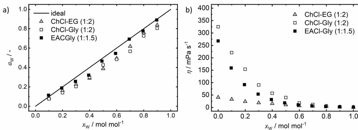
**Figure S5.** (a) Experimentally determined thermodynamic water activity of mixtures with ChCl-Gly (1:2), ChCl-EG (1:2), and EACl-Gly (1:1.5) in dependency of the water mole fraction ( $x_w$ ). (b) Experimentally measured viscosity of ChCl-Gly (1:2), ChCl-EG (1:2), and EACl-Gly (1:1.5) mixtures with water in dependency of the water mole fraction ( $x_w$ ). The activity and viscosity values for ChCl-Gly (1:2) and ChCl-EG (1:2) were taken from Bittner *et al.* [*J. Chem. Theory Comput.* 2021].
