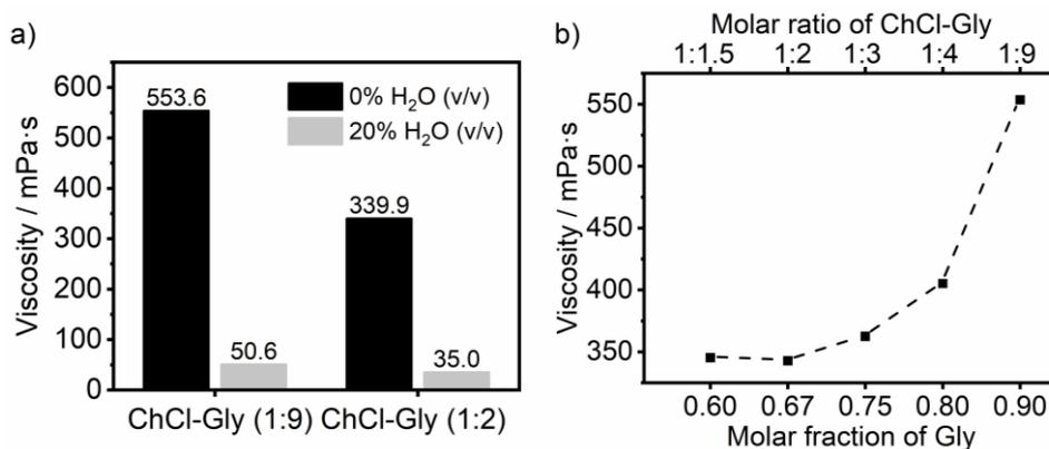
**Figure S4.** Experimentally measured viscosity of (a) ChCl-Gly (1:2) and ChCl-Gly (1:9) as pure DESs and in mixtures with 20 vol.% water and (b) ChCl-Gly with different molar ratio of ChCl:Gly.
