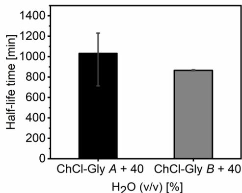
**Figure S2.** Comparison of half-life time of HLADH in ChCl-Gly (1:2) A and ChCl-Gly (1:2) B with 40 vol.% water at 60 °C.
