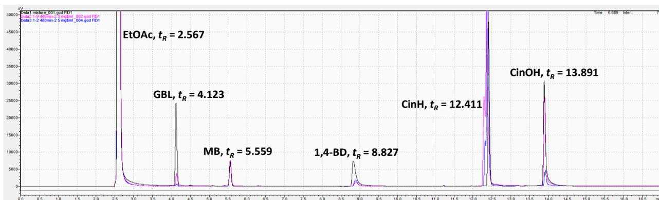
**Figure S6.** Representative GC chromatogram of components in cinnamaldehyde reduction system. (Black: mixture of all standards; blue: reaction in ChCl-Gly (1:2) with 20 vol.% water after 8 h; pink: reaction in ChCl-Gly (1:9) with 20 vol.% water after 8 h).
