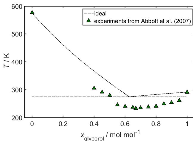
**Figure S7.** Phase diagram of eutectics at different glycerol mole fractions. ChCl: Gly (1:1.5,  $X_{Gly}$  0.6 mol mol<sup>-1</sup>; 1:2,  $X_{Gly}$  0.66 mol mol<sup>-1</sup>; 1:9,  $X_{Gly}$  0.9 mol mol<sup>-1</sup>) shows DES characteristics. Abbott et al. *Green Chem.*, 2007, 9, 868–872; DOI: 10.1039/B702833D.
