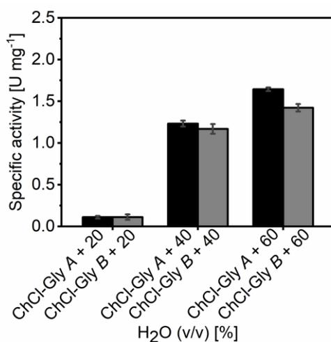
**Figure S3.** Comparison of specific activity of HLADH-catalyzed reduction in ChCl-Gly (1:2) A and ChCl-Gly (1:2) B with 20, 40, and 60 vol.% water.
