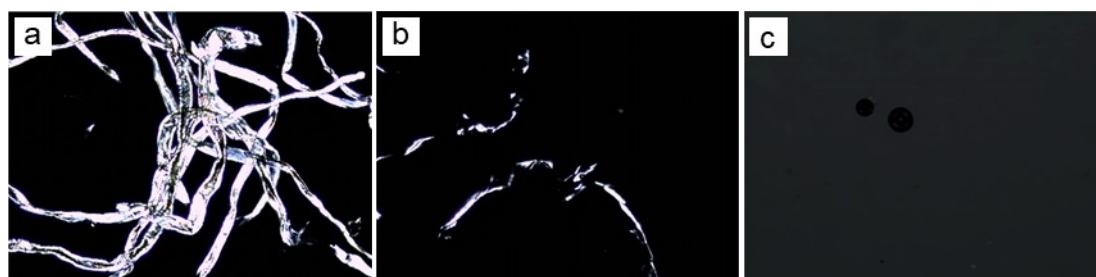
Figure S3. POM images of cellulose (DP = 926, 1 wt.)/ChOH/Urea mixture stirring at 70°C for (a) 0 min, (b) 5 min and (c) 10 min.
