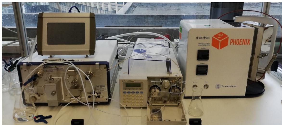
**Figure S1:** H-Cube Pro equipped with a Phoenix reactor from ThalesNano.
