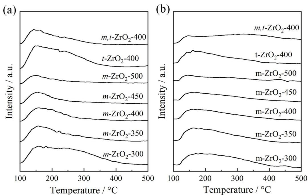
**Fig. S4** (a) CO<sub>2</sub>- and (b) NH<sub>3</sub>-TPD of *m*-ZrO<sub>2</sub>-T catalysts.
