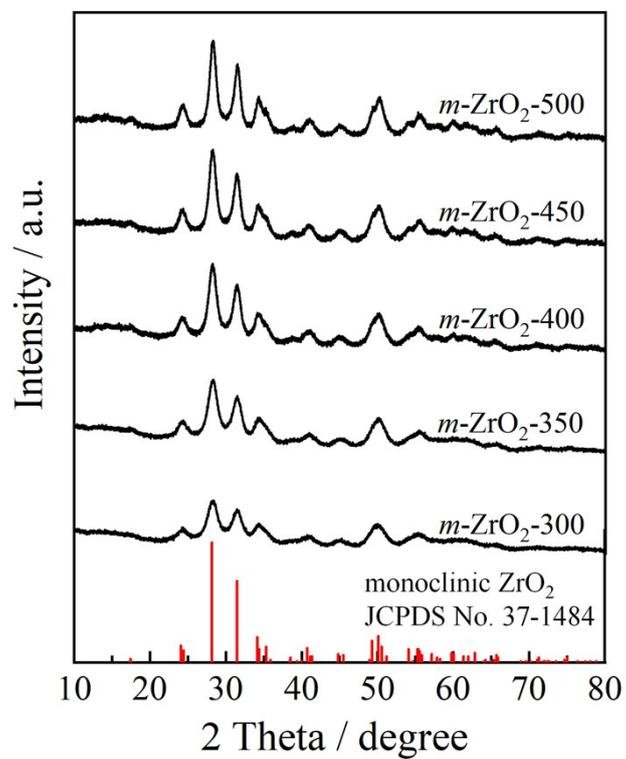
**Fig. S1** XRD patterns of *m*-ZrO<sub>2</sub> samples calcined at different temperatures in the range of 300-500 °C.
