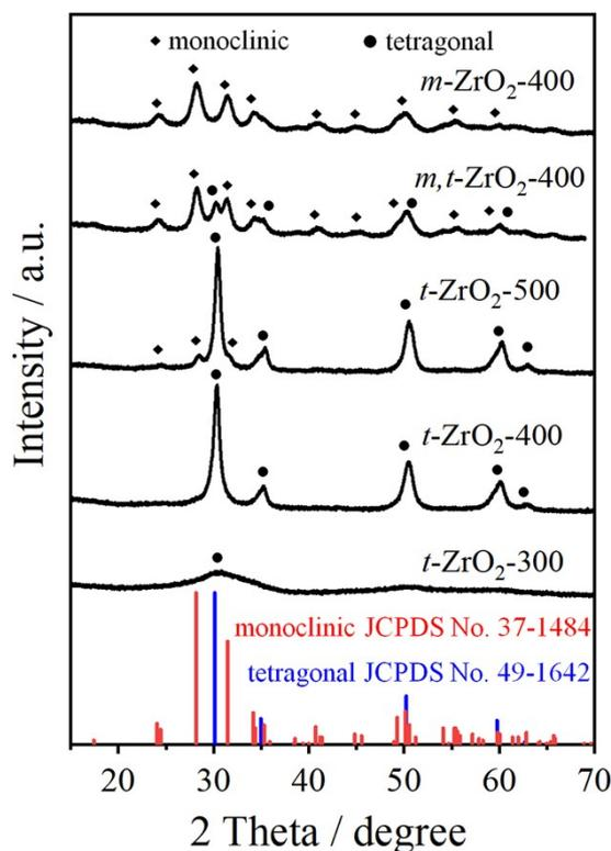
**Fig. S3** XRD patterns of  $m\text{-ZrO}_2\text{-400}$ ,  $m,t\text{-ZrO}_2\text{-400}$ ,  $t\text{-ZrO}_2\text{-300}$ ,  $t\text{-ZrO}_2\text{-400}$ , and  $t\text{-ZrO}_2\text{-500}$ .
