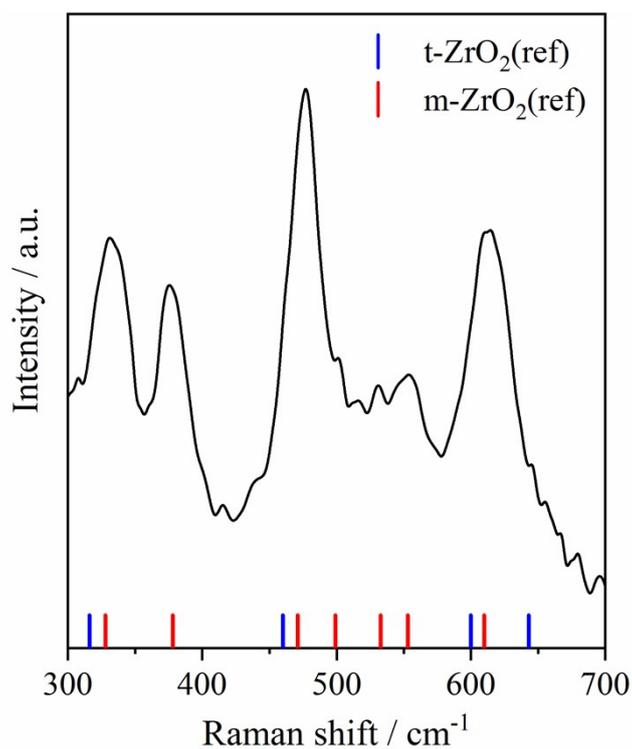
**Fig. S2** Raman spectrum for  $m\text{-ZrO}_2\text{-300}$ .
