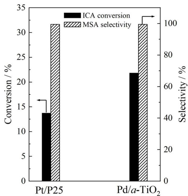
**Fig. S6** Comparison of activity of Pt/P25 and Pd/a-TiO<sub>2</sub> in the hydrogenation of ICA. Reaction condition: 5 mmol ICA, 0.05 g catalyst, 20 mL water, 2 MPa H<sub>2</sub>, 25 °C, 10 min. ICA: itaconic acid; MSA: 2-methylsuccinic acid.
