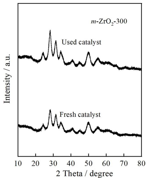
**Fig. S5** XRD patterns of  $m\text{-ZrO}_2\text{-300}$  before and after five consecutive cycles in the conversion of citric acid to ICA. Reaction conditions: 1 mmol citric acid, 0.3 g  $m\text{-ZrO}_2\text{-300}$ , 20 mL water, 2 MPa  $\text{N}_2$ , 180 °C, 40 min. ICA: itaconic acid.
