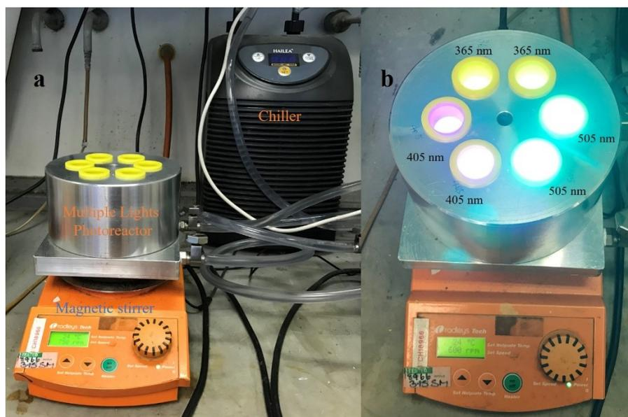
Figure S2. Multi-wavelength photoreactor.
