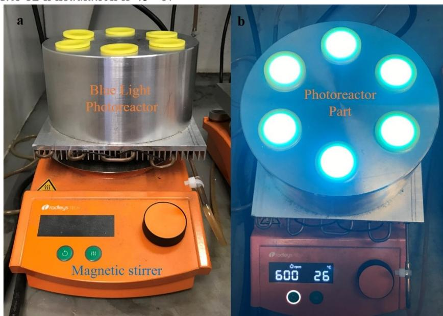
Figure S1. Blue light photoreactor.
