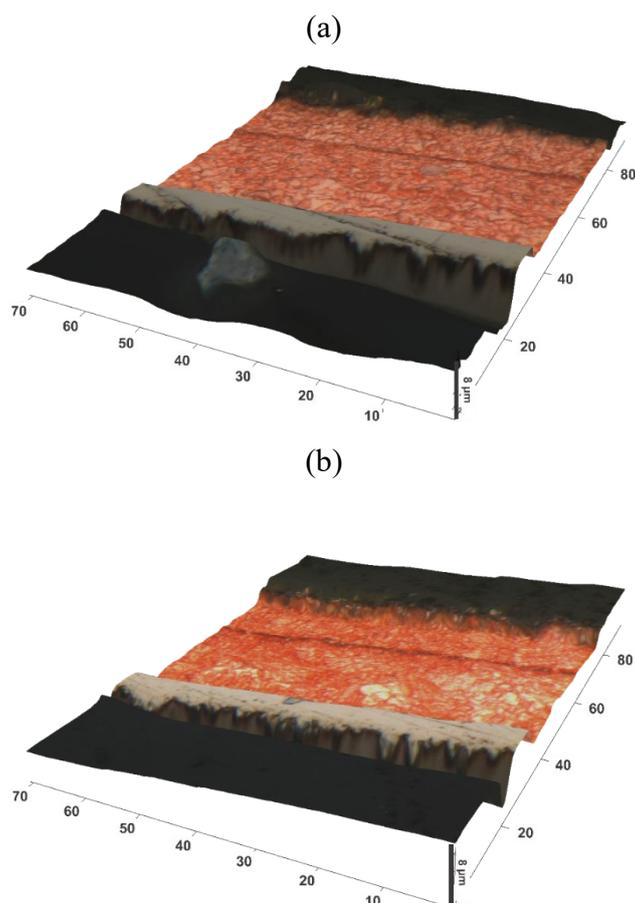
Figure S6: 3D reflected light image of the cross section of a printed circuit board block terminal with (a)  $0.02 \text{ mol dm}^{-3} \text{ CuCl}_2$  and (b)  $0.01 \text{ mol dm}^{-3} \text{ FeCl}_3$  in  $\text{CaCl}_2 \cdot 6\text{H}_2\text{O} : \text{EG}$  (1:1 ratio), for 1 hour at  $50^\circ\text{C}$ . The reddish-brown area describes the copper layer and, the white-greyish area describes the nickel layer. The dark area corresponds to the resin holding the printed circuit board sample.
