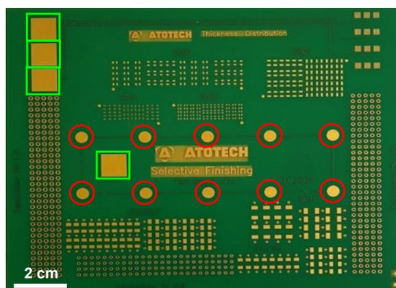
Figure S1: Gold-coated printed circuit board with block terminals of circular (in red circles) and square (in green squares)-shaped geometries.
