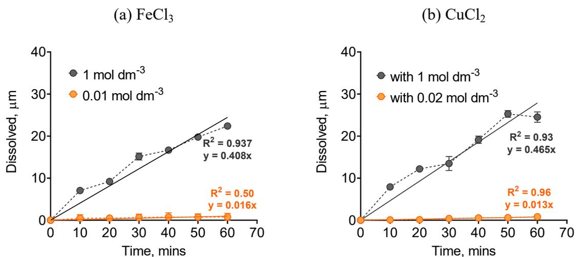
Figure S5: Etch depth of copper over time from the cross section of a square-shaped block terminal with two different concentrations of (a)  $\text{FeCl}_3$  and (b)  $\text{CuCl}_2$  as oxidising agents in the  $\text{CaCl}_2 \cdot 6\text{H}_2\text{O} : \text{EG}$  eutectic system at  $25^\circ\text{C}$ . The corresponding trend lines are also shown.
