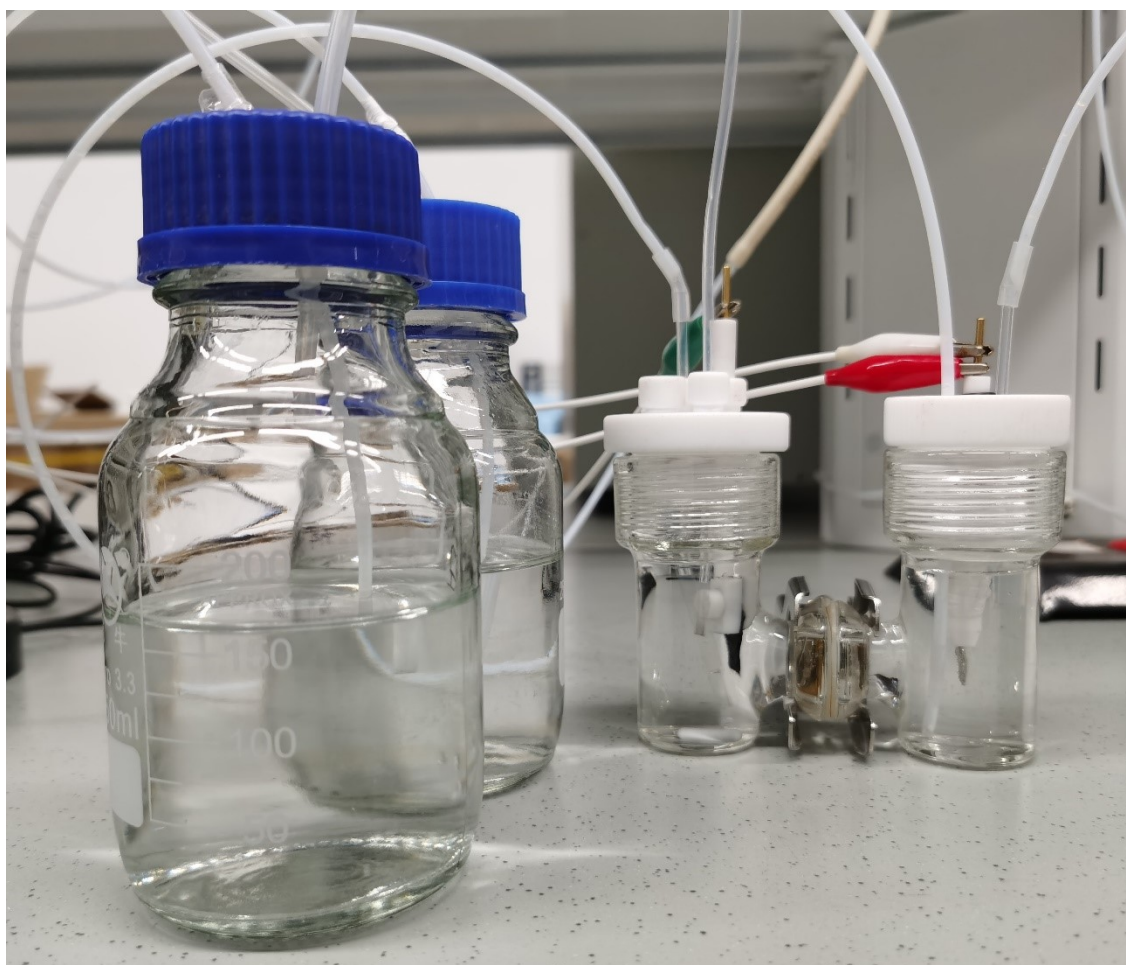
Fig. S20. Photograph of the flow reactor experiment for further stability test. The 200 mL of electrolyte was circulated through the H-cell at 70 mL/min using peristaltic pumps (Lead Fluid BT100S-1).
