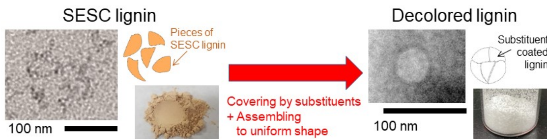
Fig. S8 | Predicted schematic illustration of the whitened mechanism of SESC lignin. Covering by substituent ( i.e. , suppression of light absorption), blocking of phenolic hydroxy groups ( i.e. , diminishing quinoid structure), and assembling to uniform shape ( i.e. , the reflection of light) would induce whitening SESC lignin nanoparticles.
