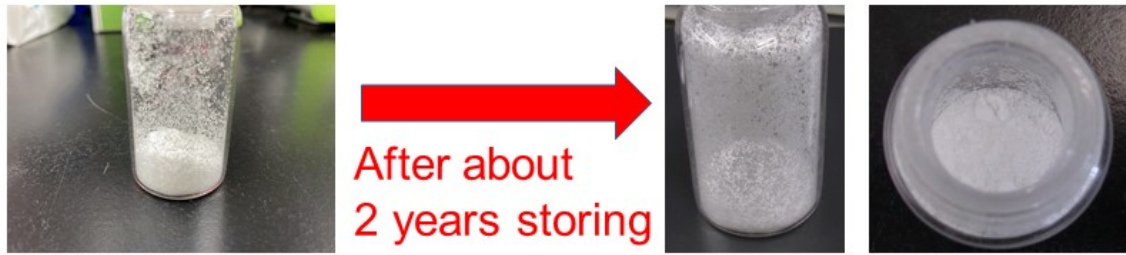
Fig. S13 | Photographs of powders of hexyl modified SESC lignin (left) before and (right) after about 2 years storing.
