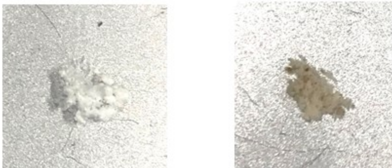
Fig. S14 | Photographs of powders of dodecyl modified SESC lignin (left) and dodecyl modified Kraft lignin (right).
