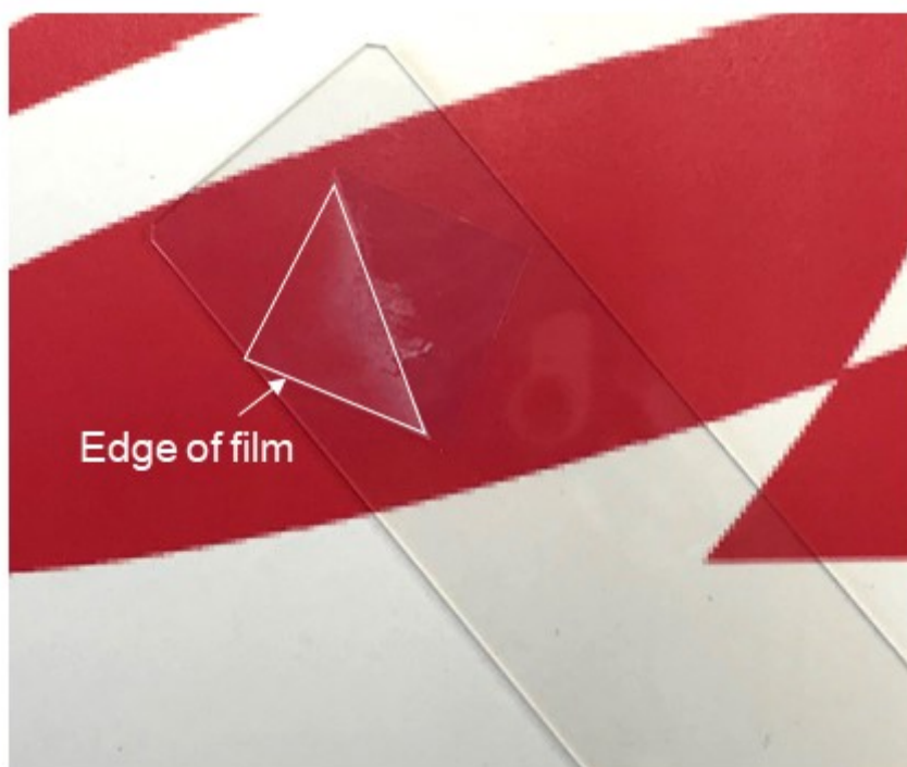
Fig. S18 | Photographs of the transparent film consisting of dodecyl modified SESC lignin obtained by hot melting that is sandwiched between two glass plates.
