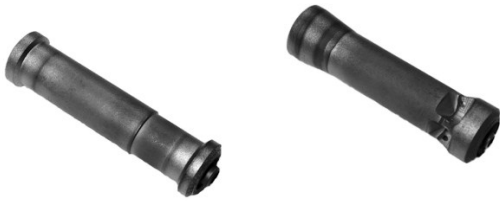
Figure S3 Comparison of different types of graphite tubes. Left: "slimmed tube"; Right: "ETV tube improved". This type was always used in this work.
