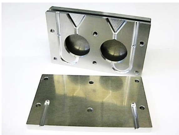
Fig. S 1 Aluminium mold used to cast EP and UP samples, 40 mm diameter cavities, a) mold open, b) mold closed.
