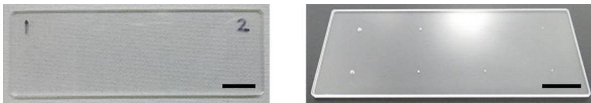
**Fig. S3** Photographs of soda-lime glass plates (left) and fused silica plates (right) after detergent treatment and glass-glass bonding. The black bars indicate 1 cm.
