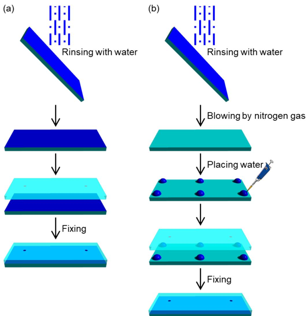
**Fig. S1** Two procedures of the described wet glass-glass bonding method. (a) Whole-surface wet bonding procedure. (b) Water-droplet bonding procedure.
