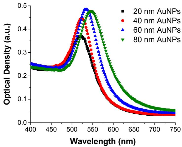
**Figure S1.** UV-Vis spectra of 20, 40, 60 and 80 nm AuNPs, with maximum absorbance peaks at 520 nm (black squares), 524 nm (red dots), 534 nm (upwards blue triangles), and 546 nm (downwards green triangles), respectively.
